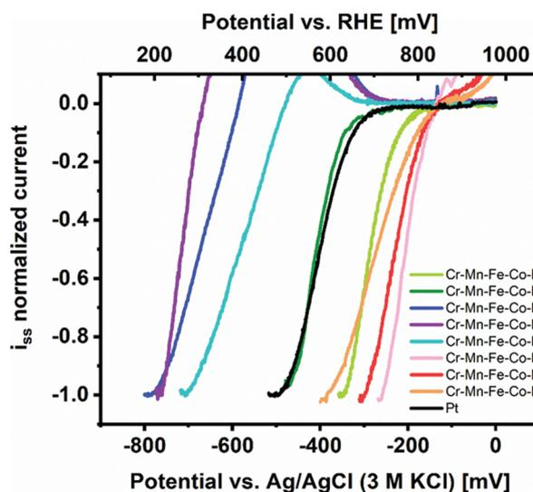
Fig. 2 Comparison of intrinsic ORR activity in alkaline media of CSSNPs immobilized on etched carbon nanoelectrodes from ILs 1 to 8 in comparison to Pt NPs.
