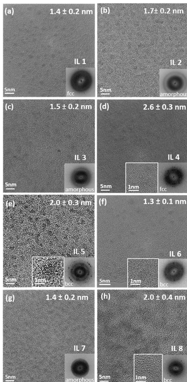
**Fig. 3** HRTEM images of CSSNPs sputtered in 8 different ILs: (a) IL 1, (b) IL 2, (c) IL 3, (d) IL 4, (e) IL 5, (f) IL 6, (g) IL 7 and (h) IL 8. The insets show the zoom in on the crystalline CSSNPs and the FFT patterns with the deduced crystal structure. Amorphous, fcc or bcc CSSNPs were found depending on the IL used in the synthesis.
