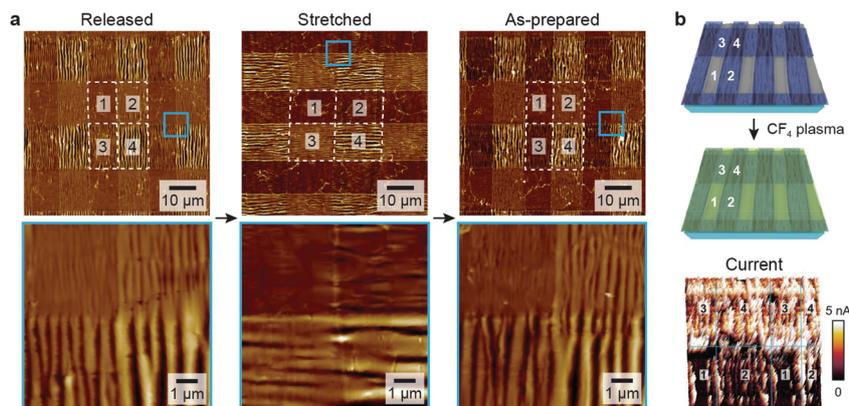
**Fig. 4** Multiscale graphene wrinkles with spatially defined structural features and properties. (a) Graphene patterned with four regions with different wavelengths. (b) Spatially defined electrical conductivities after plasma functionalization. Panel a adapted with permission from ref. 55. Copyright 2020 American Chemical Society. Panel b adapted with permission from ref. 72. Copyright 2019 American Chemical Society.
