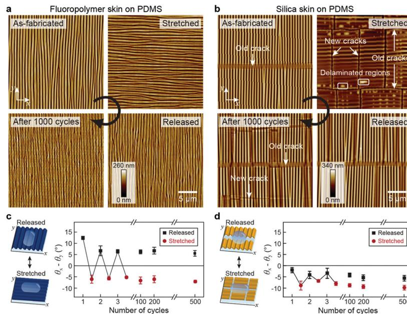
**Fig. 2** Crack-free nanowrinkles with switchable orientation enabled by plasma-mediated soft skin layers. Side-by-side comparison of wrinkle topography of (a) fluoropolymer and (b) silica skin wrinkles under stretch-release cycles. Anisotropic wetting on wrinkled (c) fluoropolymer and (d) silica skin layers. Adapted with permission from ref. 33. Copyright 2017 John Wiley and Sons.
