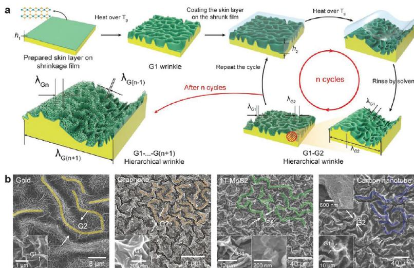
**Fig. 6** Sacrificial soft skin layers for hierarchical texturing of 2D nanomaterials. (a) Scheme illustrating the fabrication process. (b) Functional skin materials with hierarchical structures. Adapted with permission from ref. 75. Copyright 2018 American Chemical Society.
