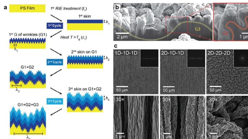
**Fig. 5** Multigenerational, hierarchical structures from sequential wrinkling of plasma-mediated soft skin layers. (a) Design principles of sequential process. (b) Conformal interface between skin layers and substrate. (c) Hierarchical wrinkles from three cycles of sequential skin growth and strain relief. Adapted with permission from ref. 34. Copyright 2015 American Chemical Society.
