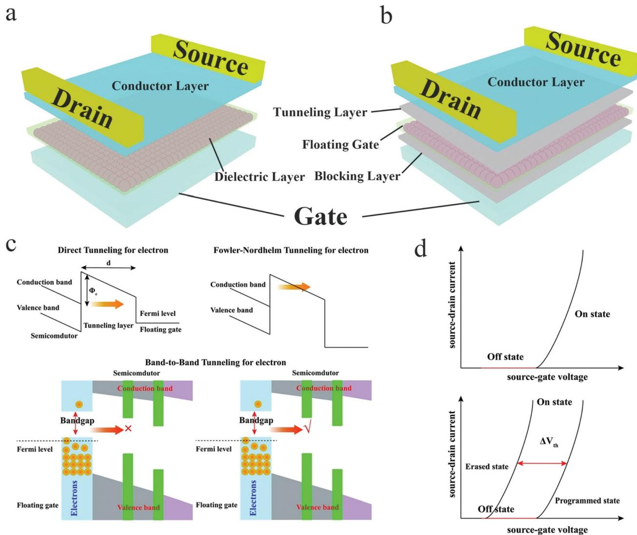
Fig. 12 (a) Schematic of an FET-based phototransistor device. (b) Schematic of a floating gate flash memory-based phototransistor device. (c) Three mechanisms of n-type flash memory device operation. (d) Transfer variation curves of the FET-based phototransistor device (top) and the floating gate flash memory-based phototransistor device (bottom).
