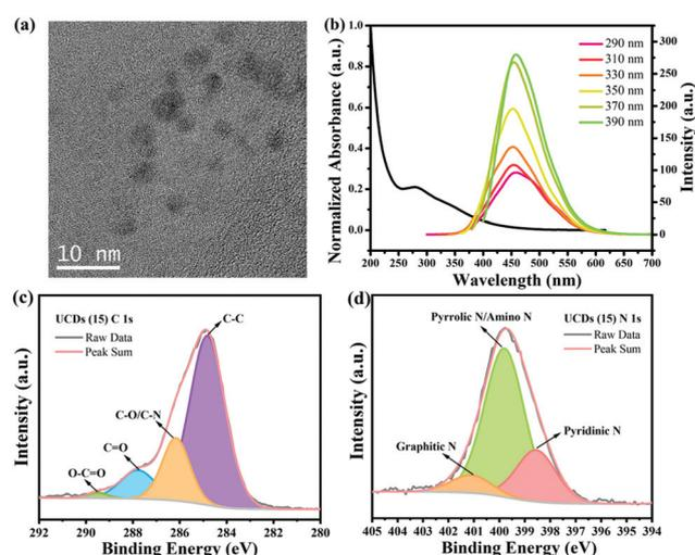
**Fig. 1** (a) TEM image of the as-prepared CDs; (b) UV-vis spectrum and PL emission spectra at various excitation wavelengths for the as-prepared CDs aqueous solution; (c) C 1s and (d) N 1s core-level spectra of UCDS (15).
