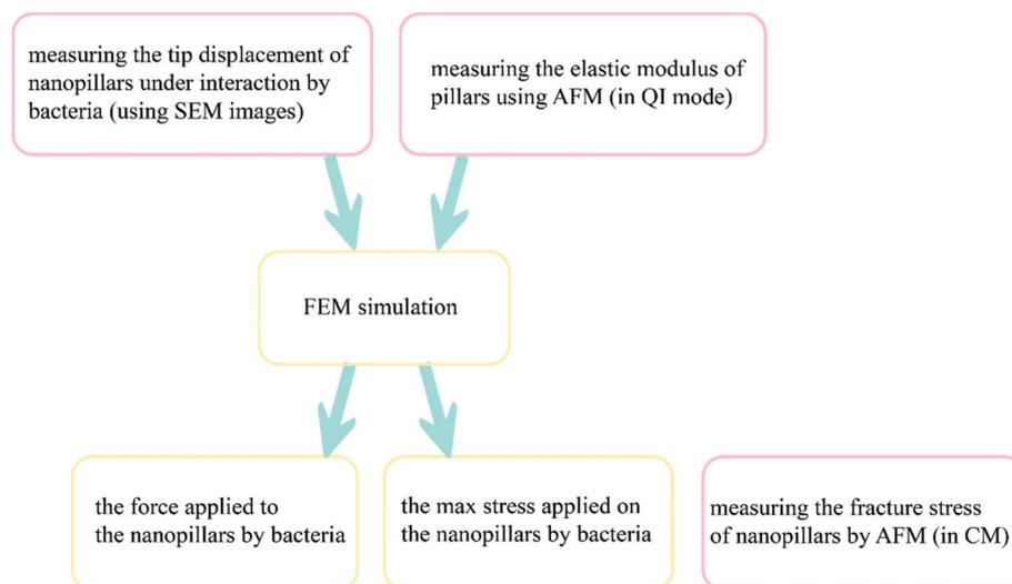
**Fig. 6** A schematic drawing illustrating the procedure used to evaluate the stress state of our EBID nanopillars and their interaction force with bacteria. Pink blocks indicate the experimentally measured parameters while the yellow blocks indicate the parameters determined by simulation.
