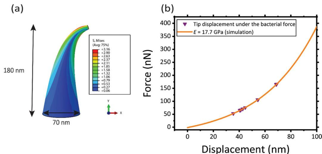
**Fig. 5** (a) A nanopillar was modeled in Abaqus to simulate the stresses experienced by the nanopillars due to the bacterial force. (b) The orange graph represents the force-displacement curve obtained through FEM (for the nanopillar with  $E = 17.7$  GPa). The displacement of the tip of the nanopillars under bacterial force was fitted in the graph (purple triangles).
