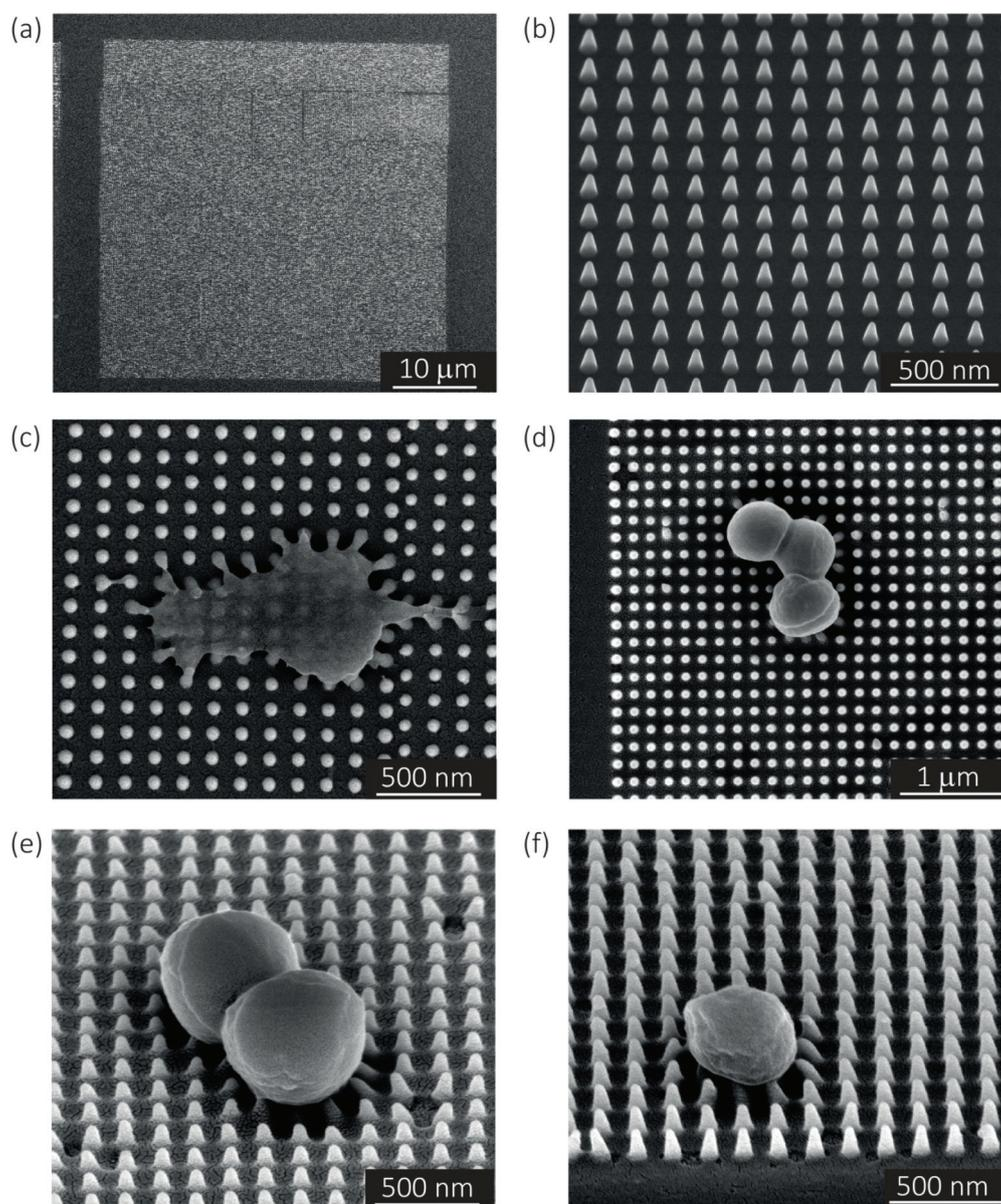
**Fig. 1** The SEM images of the nanopillars (with an average height of 180 nm, an average diameter of 70 nm, and average interspacing of 170 nm) produced by EBID at different magnifications: (a) top view and (b)  $52^\circ$ -tilted view. The SEM images of *S. aureus* bacteria on the nanopatterned surface: (c and d) the top and (e and f)  $52^\circ$ -tilted views.
