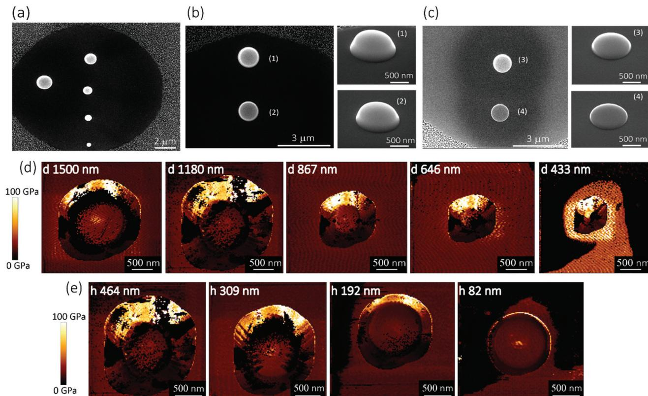
**Fig. 2** The SEM image of pillars with (a) different diameters: 433, 646, 867, 1180, and 1500 nm, (b and c) different heights: 1–464 nm, 2–309 nm, 3–192 nm, 4–82 nm. (The left figures were taken from the top view while the right figures were taken from 52°-tilted view.) (d) The map of the elastic modulus of the pillars with different diameters obtained by AFM. (e) The map of the elastic modulus of the pillars with different heights obtained by AFM.
