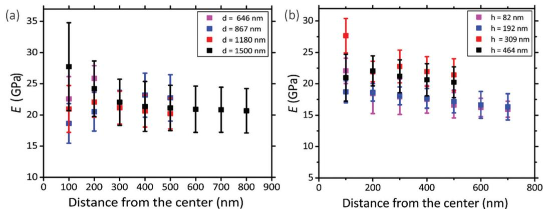
**Fig. 3** (a) The distribution of the elastic modulus for the pillars with different diameters in different distances from the center. (b) The distribution of the elastic modulus for the pillars with different heights (with the same diameter of 1000 nm) at different distances from the center. The pillars were deposited with an acceleration voltage of 17.8 kV and a current of 0.6 nA.
