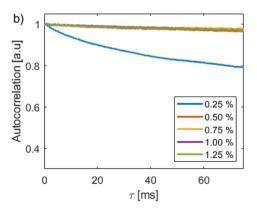
Fig. 4 Average autocorrelation curves for agarose gels ranging from 0.25% to 1.25%. (a) Autocorrelation curves for agarose gels containing nanobubbles from the same stock solution, and (b) autocorrelation curves for gels containing microbubbles from the same stock solution. The autocorrelation curves have been offset vertically to intersect the ordinate at unity. The legend in (b) is applicable to both graphs.
