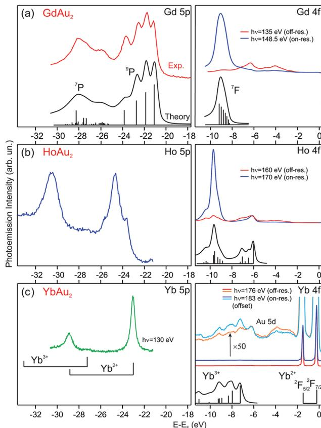
**Fig. 2** Photoemission spectra taken at  $T = 17$  K of 5p and 4f rare-earth core levels for (a)  $\text{GdAu}_2$ , (b)  $\text{HoAu}_2$ , and (c)  $\text{YbAu}_2$  monolayers grown on  $\text{Au}(111)$ . The valence state of the rare-earth atom can be determined by comparing with theoretically calculated multiplets, shown under the corresponding spectra (multiplet data reproduced from ref. 20 and 36–39).
