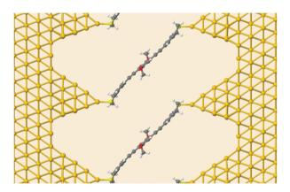
Fig. 6 Device geometry for DFTB transport simulations. Shown is OPE3-Ph(OMe)<sub>2</sub> connected to semi-infinite gold leads.
