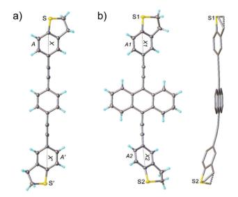
Fig. 2 X-ray molecular structures. (a) Projection on the central phenylene plane (Ph) of OPE3-Ph, inversion-related entities are primed, thermal ellipsoids are drawn at 50% probability level and (b) major conformer of OPE3-An, projection on the anthracene (An) plane, and sideview showing the disorder (H atoms omitted).
