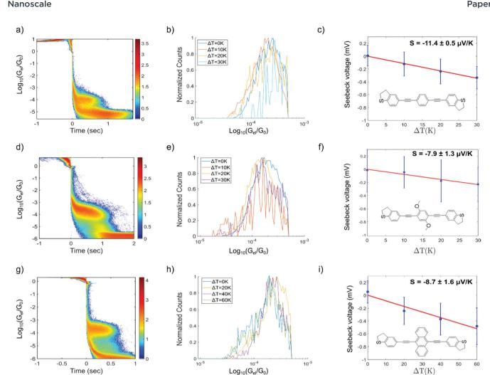
Fig. 4 Break-junction conductance histograms (a, d, and g) with a logarithmic color bar (log(counts)), 1D single-molecule conductance traces obtained as a function of the temperature (b, e and h) and Seebeck voltage vs. dT graphs (c, f and i) respectively, obtained for OPE3-Ph, OPE3-Ph(OMe)<sub>2</sub> and OPE3-An.
