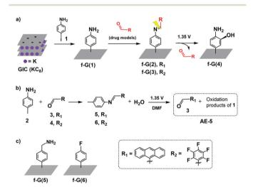
**Scheme 1** Schematics of the preparation of (a) the graphene-based platform f-G(1) loaded with the drug models (f-G(2-3)) followed by their electrochemically triggered release (f-G(4)); (b) graphene-free organic models employed to characterise the release mechanism; (c) graphene-based materials for the control experiments.
