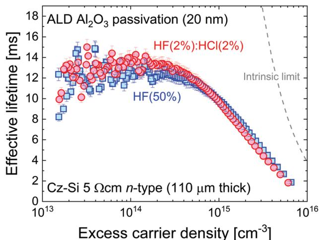
**Fig. 6** Effective lifetime versus excess carrier density for 110  $\mu\text{m}$  thick 5  $\Omega \text{ cm}$  n-type Cz-Si samples from the same wafer treated with HF(2%):HCl(2%) or HF(50%) for 10 min immediately before the ALD process (200 °C deposition with 460 °C activation). The level of surface passivation is the same within the 5% error shown, unlike for the superacid-derived passivation in Fig. 1(b). The intrinsic lifetime limit from Richter *et al.*<sup>23</sup> is also shown.
