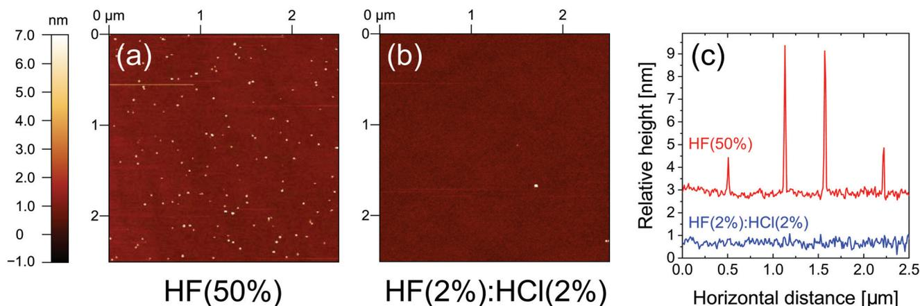
**Fig. 5** Representative 25 μm × 25 μm AFM maps of 5 Ω cm n-type FZ-Si after (a) an HF(50%) treatment for 10 min and (b) an HF(2%):HCl(2%) treatment for 10 min. Neither sample had been subsequently treated with superacid-derived passivation. The horizontal line scans in (c) show scans typical of both sample types.
