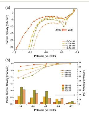
Fig. 3 CO<sub>2</sub>RR performance analysis (a) LSV measurements of O-Zn-200, O-Zn-300, O-Zn-400 and O-Zn-500. Partial current density (up in b) and faradaic efficiency (bottom in b) of formate of O-Zn-200, O-Zn-300, O-Zn-400 and O-Zn-500 in a selected potential window of 0.70 to -1.10 V (vs. RHE).
