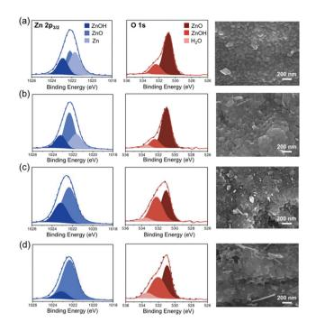
Fig. 2 Fitting results of Zn  $2p_{3/2}$  and O 1s XPS spectra and corresponding SEM images for (a) O-Zn-200, (b) O-Zn-300, (c) O-Zn-400 and (d) O-Zn-500 samples.
