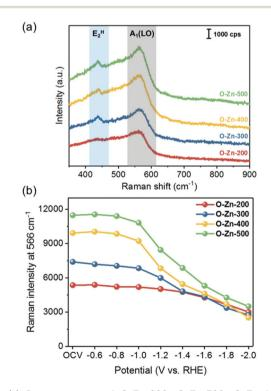
Fig. 4 (a) Raman spectra of O-Zn-200, O-Zn-300, O-Zn-400 and O-Zn-500, and (b) their peak intensity at 566 cm<sup>-1</sup> based on in situ Raman monitoring
