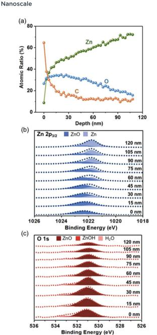
Fig. 1 Depth analysis of pristine Zn foil. (a) Quantification of elemental analysis from XPS. Fitting results of XPS spectra as a function of depth for (b) Zn  $2p_{3/2}$  and (c) O 1s.
