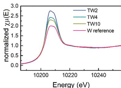
Fig. 5 W L<sub>3</sub>-edge XANES spectra of three W-doped TiO<sub>2</sub> and W-reference samples.
