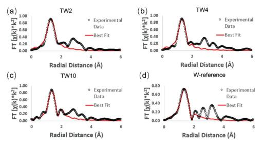
Fig. 6 W L<sub>3</sub>-edge FT-EXAFS spectra of different samples: (a) TW2, (b) TW4, (c) TW10, and (d) W-reference.
