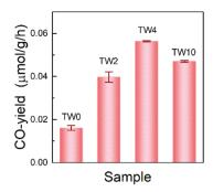
Fig. 3 Photothermocatalytic-induced CO<sub>2</sub> conversion over TW0. TW2. TW4 and TW10.
