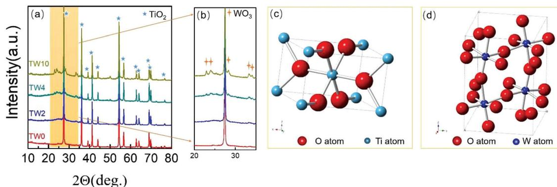
Fig. 2 (a) XRD patterns and (b) magnified XRD patterns in the region of 20–35 degrees of TW0, TW2, TW4 and TW10. (c) TiO<sub>2</sub> and (d) WO<sub>3</sub> unit cell images.
