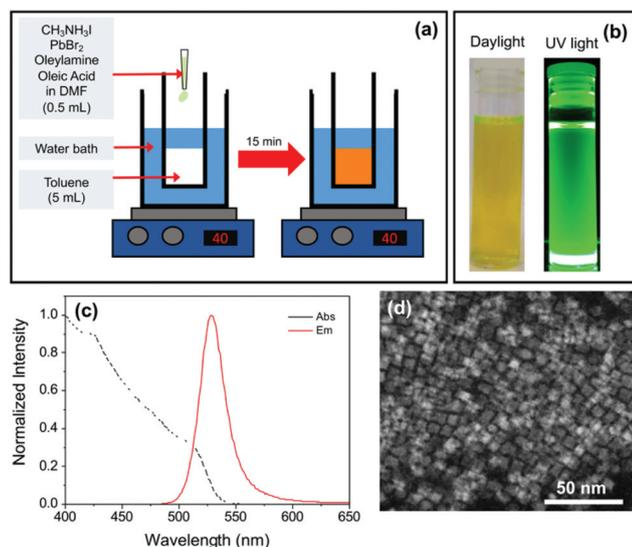
**Fig. 1** Fabrication and characterisation of a standard sample of  $\text{MAPbBr}_{3-x}\text{I}_x$  PNCs in toluene. (a) Scheme of the LARP synthesis protocol. (b) Photographs of the PNC suspension obtained after centrifugation under white (left) and UV (right) illumination. (c) UV/Vis absorption (black dashed line) and steady-state photoluminescence (red solid line) spectra ( $\lambda_{\text{ex}} = 400 \text{ nm}$ ). (d) STEM image revealing the formation of platelets.
