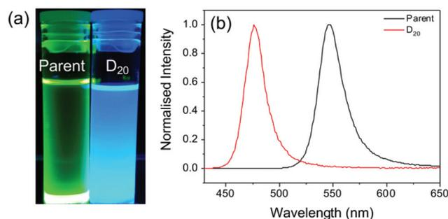
**Fig. 3** MAPbBr<sub>3-x</sub>I<sub>x</sub> PNC dispersions show different optical properties upon dilution in a more polar solvent (chloroform). (a) Photographs of the dispersion before and after dilution D<sub>20</sub> under illumination at 365 nm and (b) corresponding PL spectra ( $\lambda_{\text{ex}} = 400$  nm).
