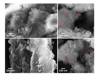
Fig. 9 SEM micrographs of (a and b)  $Pt-Cu-Se_B/g-C_3N_4$  and, (c and d)  $Pt-Cu-Se_C/g-C_3N_4$  nanocomposites. Red circles indicate the position of  $Pt-Cu-Se_X$  NPs
