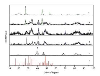
Fig. 2 XRD patterns of (a)  $Cu_{2-x}Se$  NPs, (b) sample A (ratio Pt: Cu 0.1), (c) sample B (ratio Pt: Cu 0.2), (d) sample C (ratio Pt: Cu 0.65) and, (e) sample D (ratio Pt: Cu 1.6). Reference patterns of cubic  $Cu_2Se$  (JCPDS 088-2043) in green; cubic CuPt (JCPDS 048-1549) in blue; cubic Pt (JCPDS 087-0640) in black, and monoclinic  $Pt_5Se_4$  (JCPDS 00-031-0950) in red.
