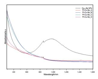
Fig. 8 UV-Vis-NIR absorption spectra of  $Cu_{2-x}Se$  and  $Pt-Cu-Se\_A-D$  samples.
