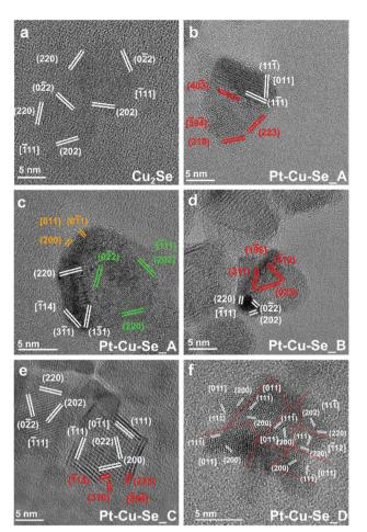
Fig. 7 HRTEM images of representative NPs of Cu<sub>2</sub>Se (panel a), Pt-Cu-Se\_A (panels b and c), Pt-Cu-Se\_B (panel d), Pt-Cu-Se\_C (panel e), Pt-Cu-Se\_D (panel f). Different phases in panels B-E are depicted in false colors as indicated: phase A (main)  $\rightarrow$  white; phase B (main)  $\rightarrow$ red, phase A (minor)  $\rightarrow$  green; phase B (minor)  $\rightarrow$  orange.
