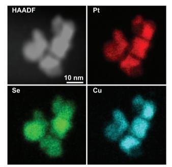
**Fig. 5** HAADF-STEM image and corresponding elemental maps by STEM EDS of Pt-Cu-Se\_C.
