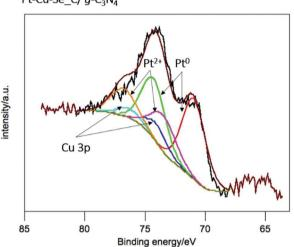
Fig. 10 X-ray photoelectron spectra of the Pt 4f core level for Pt-Cu- $Se_B/g-C_3N_4$  and  $Pt-Cu-Se_C/g-C_3N_4$  nanocomposites, and corresponding deconvolutions.
