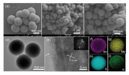
Fig. 4 (a) SEM image of the MoG nanospheres; (b and c) SEM images of the MoS<sub>2</sub>@SnS heterostructures with different magnifications; (d) TEM image of the MoS<sub>2</sub>@SnS heterostructures; (e) HRTEM image of the MoS<sub>2</sub>@SnS heterostructures with the corresponding fast Fourier transform (FFT) pattern (inset); EDS elemental mapping of (f) Sn, (g) Mo, (h) S and (i) N elements in the MoS<sub>2</sub>@SnS composite.
