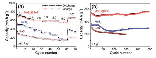
Fig. 6 (a) Rate capability and (b) cycling stability of the SnS microflowers, MoS<sub>2</sub> nanospheres and MoS<sub>2</sub>@SnS heterostructures at the indicated densities.
