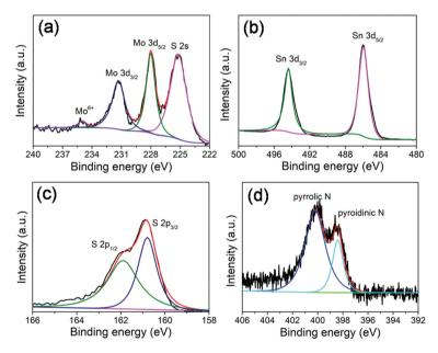
Fig. 3 High-resolution XPS spectra of the MoS<sub>2</sub>@SnS heterostructure. (a) Mo 3d; (b) Sn 3d; (c) S 2p; and (d) N 1s spectra.
