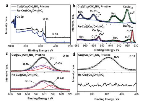
Fig. 2 (a) XPS survey spectra and high-resolution XPS spectra of (b) Cu 2p, (c) O 1s, and (d) N 1s of the  $Cu@Cu_2(OH)_3NO_3$  electrode before and after pre-reduction.
