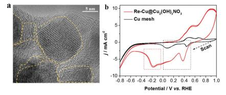
Fig. 5 (a) HRTEM image of the Re-Cu@Cu<sub>2</sub>(OH)<sub>3</sub>NO<sub>3</sub> nanodendrite and (b) cyclic voltammograms of the Re-Cu@Cu<sub>2</sub>(OH)<sub>3</sub>NO<sub>3</sub> and bare Cu mesh electrodes in 0.1 M KHCO<sub>3</sub> (saturated with Ar) for four segments respectively, without stirring, scan rate: 20 mV s<sup>-1</sup>.
