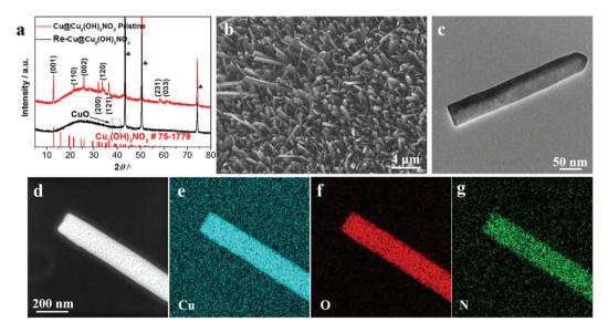
Fig. 1 (a) XRD patterns of the Cu@Cu<sub>2</sub>(OH)<sub>3</sub>NO<sub>3</sub> electrode before (red) and after (black) pre-reduction, (b) SEM and (c) TEM images of the pristine Cu@Cu2(OH)3NO3 electrode, (d) HAADF-STEM image and the corresponding elemental mapping images of (e) Cu, (f) O, and (g) N.
