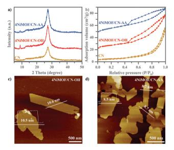
Fig. 1 XRD patterns (a) and N<sub>2</sub> sorption isotherm curves (b) from CN, 4NiMOF/CN-OH and 4NiMOF/CN-AA. AFM images of 4NiMOF/CN-OH (c) and 4NiMOF/CN-AA (d).
