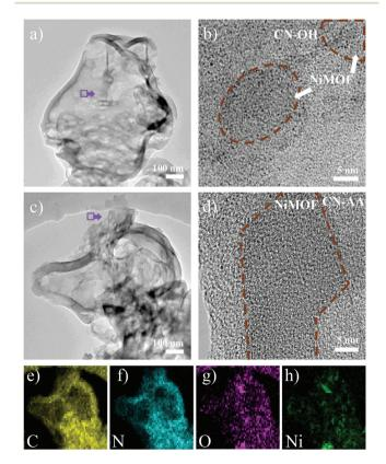
Fig. 2 TEM (a) and HRTEM (b) images of 4NiMOF/CN-OH. TEM (c), HRTEM (d) and elemental mapping images (e-h) of 4NiMOF/CN-AA.
