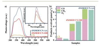
Fig. 4 SS-SPS responses and FS spectra (inset) related to the amount of produced 'OH (a) and the photocatalytic activities for  $CO_2$  conversion under visible-light irradiation for 4 hours (b) of CN, 4NiMOF/CN-OH and 4NiMOF/CN-AA.
