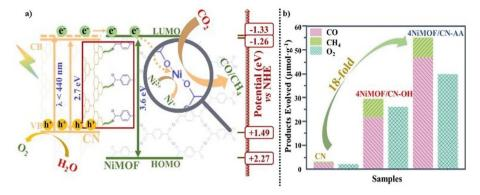
Fig. 6 (a) A schematic diagram of the photogenerated charge transfer process and the induced photochemical reaction in the resultant NiMOF/ functionalized CN nanocomposite. (b) Photocatalytic activities for CO2 conversion under UV-vis irradiation for 4 hours of CN, 4NiMOF/CN-OH and 4NiMOF/CN-AA.
