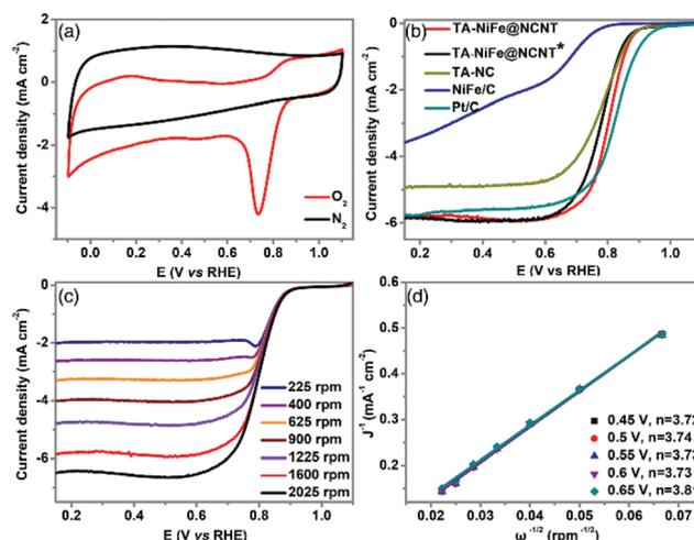
Fig. 4 (a) CV curves for TA-NiFe@NCNT in O<sub>2</sub> and N<sub>2</sub> saturated 0.1 M KOH electrolytes collected at a scan rate of 100 mV s<sup>-1</sup>. (b) ORR LSV curves for TA-NiFe@NCNT, TA-NiFe@NCNT\*, TA-NC, NiFe/C, and Pt/C collected at a rotation speed of 1600 rpm and a scan rate of 10 mV s<sup>-1</sup>. (c) ORR LSV curves for TA-NiFe@NCNT at various rotation speeds. (d) K-L plots for TA-NiFe@NCNT at different potentials derived from the corresponding ORR LSV curves.
