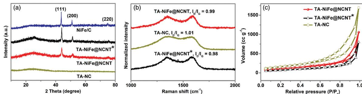
Fig. 2 (a) XRD patterns for TA-NiFe@NCNT, TA-NiFe@NCNT\*, TA-NC, and NiFe/C. (b) Raman spectra, and (c) N<sub>2</sub> adsorption and desorption isotherms of TA-NiFe@NCNT, TA-NiFe@NCNT\*, and TA-NC.
