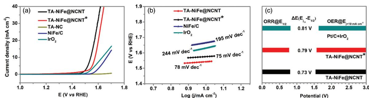
Fig. 5 (a) OER LSV curve for various catalysts at a scan rate of  $5 \text{ mV s}^{-1}$  and a rotation speed of 1600 rpm after 95%-*iR* correction. (b) Tafel plots derived from the corresponding OER LSV curves. (c) The potential gap ( $\Delta E$ ) between the OER potential measured at a current density of  $10 \text{ mA cm}^{-2}$  and the ORR half-wave potential.
