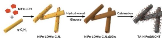
**Scheme 1** Schematic illustration of the preparation process of TA-NiFe@NCNT.
