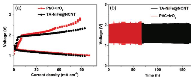
Fig. 6 (a) Charge and discharge polarization curves of rechargeable zinc-air batteries. (b) Charge and discharge cycling curves of rechargeable zinc-air batteries at a current density of  $25 \text{ mA cm}^{-2}$ .
