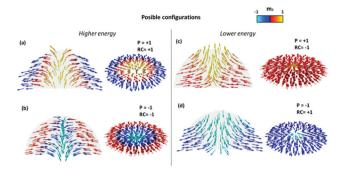
Cross section and basal planes of the dome shaped nanodots, showing possible magnetic configurations with radial magnetic anisotropy, combining positive and negative core polarities and inwards and outwards radial magnetization. The energy of the configurations in (a) and (b) are 13% higher than those in (c) and (d). P stands for Polarity and RC for radial chirality.
