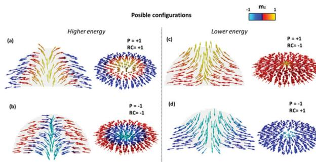
**Fig. 2** Cross section and basal planes of the dome shaped nanodots, showing possible magnetic configurations with radial magnetic anisotropy, combining positive and negative core polarities and inwards and outwards radial magnetization. The energy of the configurations in (a) and (b) are 13% higher than those in (c) and (d). *P* stands for Polarity and *RC* for radial chirality.
