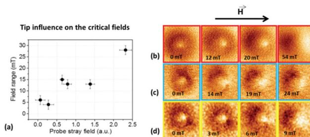
**Fig. 5** Assessment of the half-hedgehog stability as a function of the magnetic force gradient. (a) Correlation between OOP magnetic probe stray field (x axis) and the field range where the structure is stable (y axis). The black dots represent the experimental data obtained from the MFM based measurements described in ESI7.† Field sequences performed with different tips show the decreasing saturating in-plane magnetic fields from (b)–(d). Image size is 250 × 250 nm.
