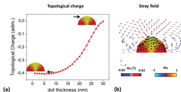
**Fig. 4** (a) 2D topological charge versus the thickness coordinate of the dot. (b) Simulated stray field of the dome-shaped nanodot. Black arrows represent the magnetization following stream lines. Red-Grey-blue arrows show the field direction (unitary vector) and the colour the Hz component of magnetization over the base of the dot.
