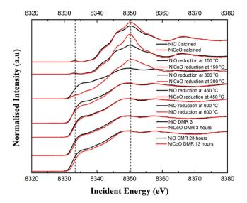
Fig. 5 Ni Kβ-detected HERFD XAS spectra of NiO/ $\gamma$ -Al<sub>2</sub>O<sub>3</sub> and NiCoO/ $\gamma$ -Al<sub>2</sub>O<sub>3</sub> collected for the freshly calcined samples, during the reduction/activation step, and under DMR conditions. The pre-edge and main edge peak positions have been indicated with dashed lines.
