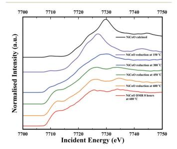
Fig. 6 Co Kβ-detected HERFD spectra of the NiCoO/ $\gamma$ -Al<sub>2</sub>O<sub>3</sub> sample measured under ambient, reduction activation (5% H<sub>2</sub> in Ar), and DMR (7% CH<sub>4</sub> and 9.5% CO<sub>2</sub> diluted in N<sub>2</sub>) conditions.
