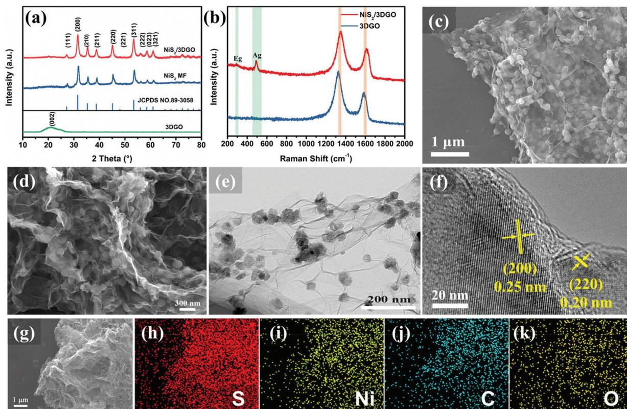
Fig. 2 (a) XRD comparison of NiS<sub>2</sub>/3DGO, NiS<sub>2</sub> MF and 3DGO; (b) Raman spectrum of NiS<sub>2</sub>/3DGO and 3DGO; (c and d) Representative SEM images of NiS<sub>2</sub>/3DGO; (e and f) TEM and HRTEM images of NiS<sub>2</sub>/3DGO; (g–k) SEM images and corresponding elemental mapping analysis of NiS<sub>2</sub>/3DGO.
