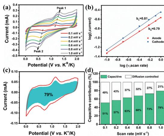
Fig. 5 (a) CV curves of  $NiS_2/3DGO$  at scan rates range from 0.1 to  $1.0\text{ mV s}^{-1}$ . (b) Linear relationship of  $\log(i)$  vs.  $\log(v)$ . The contribution ratio of the capacitive capacities and diffusion-limited capacities at  $1\text{ mV s}^{-1}$  (c) and at different scan rates (d).
