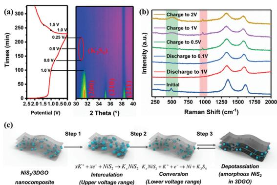
**Fig. 6** (a) *In situ* XRD results of NiS<sub>2</sub>/3DGO during the first cycle at the cut-off voltage of 0.01–2.0 V. (b) *Ex situ* Raman spectrum of NiS<sub>2</sub>/3DGO at different discharged/charged states. (c) Schematic illustration of the potassium storage mechanism.
