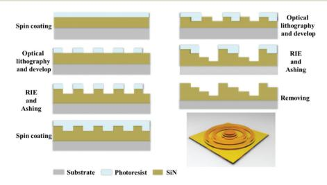
Fig. 3 The 4-inch wafer-level fabrication flow for the step-shaped MPM SOLs.
