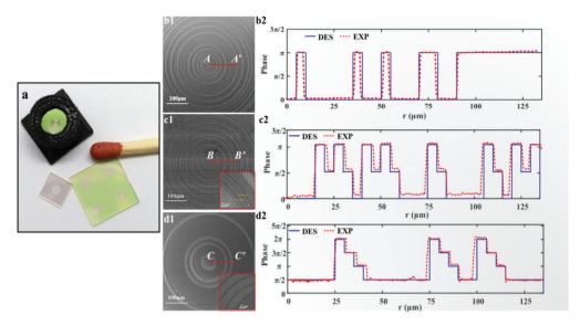
Fig. 4 The device images obtained by both SEM and a step profiler for the three fabricated MPM SOLs. (a) The device image of the MPM SOLs; (b1, c1, d1) The SEM images for the three samples; (b2, c2, d2) The cross-sectional views of the as-fabricated SOLs' geometrical profiles radially for the three samples.
