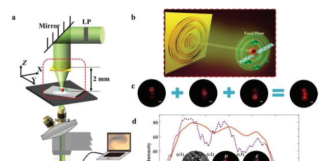
Fig. 7 (a) Schematic of imaging measurement setup for the dispersive fluorescent particles. LP: Linear Polarizer. (b) Illustrative diagram for imaging the fluorescent particles. (c) Superposition operation of the achieved images. (d) The imaging results of fluorescent nanoparticles obtained by employing bright-field microscopy, wide-field fluorescence microscopy and SOL-based microscopy, respectively. Scale bar, 1 µm.
