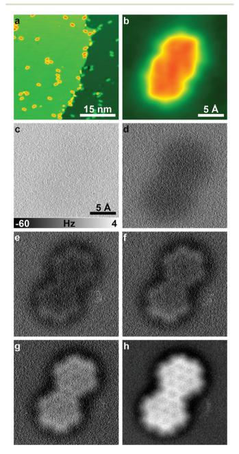
Fig. 2 (a) STM image of non-oxidized Cu(110) surface with  $\approx$ 0.1 monolayer DCLN molecules. (b) STM image of the DCLN molecule taken before AFM experiments. Height dependent CH-AFM of DCLN molecule (c) at  $\Delta z_{\rm ch}$  = 360 pm (d) at  $\Delta z_{\rm dh}$  = 240 pm (e) at  $\Delta z_{\rm eh}$  = 90 pm (f) at  $\Delta z_{\rm fh}$ = 60 pm (g) at  $\Delta z_{\rm gh}$  = 20 pm and (h) at the closest distance.
