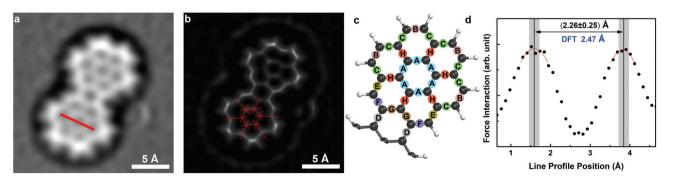
Fig. 3 (a) Image obtained at 78 K after LoG filter is applied, (b) SD filtered<sup>30</sup> image to sharpen the peripheral bonds for analysis, (c) the model showing half of the DCLN molecule, each letter representing a bond group according to their DFT lengths, (d) line profile obtained from LoG filtered image, marked by red line in (a).
