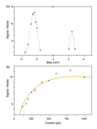
Fig. 3 Signal to noise analysis of the sensing scheme performance. (a) Signal-to-noise ratio for remote measurement of the nano-AF spin states as a function of applied DC bias. Tunnel current setpoint 300 pA. Blue dots are experimental data, the dotted lines are guides to the eye. (b) Signal-to-noise ratio as function of tunnel current setpoint with an applied DC bias -5.2 mV. Blue dots are experimental data, orange line is a fit obtained using our model (see ESI† for details).
