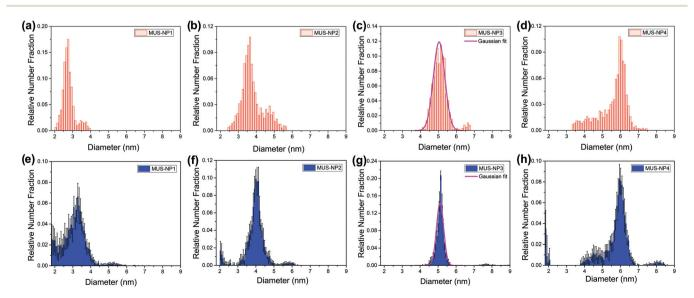
Fig. 3 Diameter distribution analysis of single-type samples by TEM (red) and SAXS (blue): (a) and (e) MUS-NP1, (b) and (f) MUS-NP2, (c) and (g) MUS-NP3, (d) and (h) MUS-NP4.
