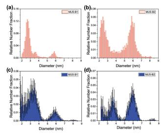
Fig. 4 Diameter distribution analysis of binary mixtures by TEM (red) and SAXS (blue): (a) and (c) MUS-B1 (1:1 wt), (b) and (d) MUS-B2 (1:5
