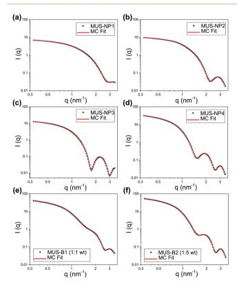
Fig. 2 SAXS profiles and MC fitting (log-log plots) of (a) 5 mg ml<sup>-1</sup> MUS-NP1, (b) 5 mg ml $^{-1}$  MUS-NP2, (c) 5 mg ml $^{-1}$  MUS-NP3, (d) 5 mg ml $^{-1}$ MUS-NP4, (e) 10 mg ml<sup>-1</sup> MUS-B1 (1:1 wt) and (f) 10 mg ml<sup>-1</sup> MUS-B2
