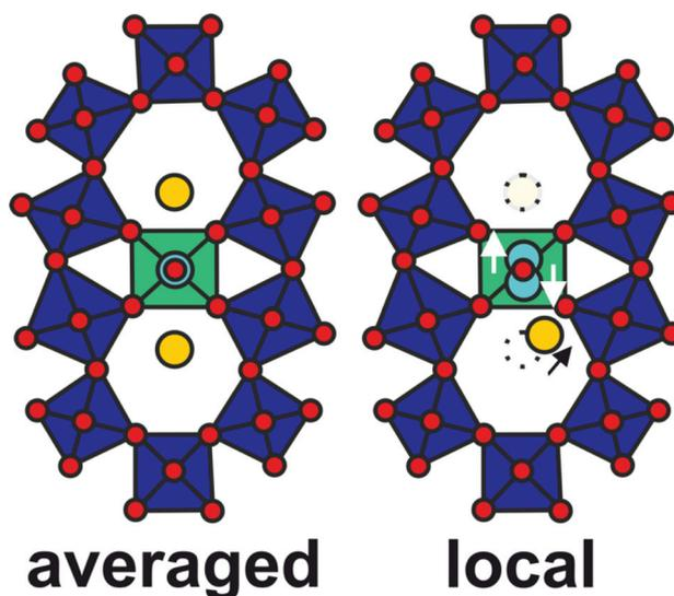
**Scheme 1** Comparison between the averaged ideal structure (left) and the observed local real structure (right) around the S2 site of  $(Mo,V,Te,Nb)O_x$ . The arrows denote the shift direction of the S2 site. Green: Oxygen polyhedra surrounding the S2 site; yellow: tellurium; red: oxygen, blue: S2 cation, dashed: un-displaced positions.
