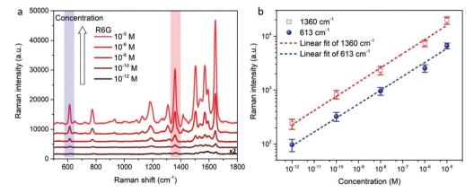
Fig. 6 (a) The Raman spectra of R6G with different concentrations adhered on the 3D-Ag-HNA SERS substrate, and in order to be clarified, the spectrum of  $10^{-12}$  M R6G was multiplied by 2 fold. (b) The SERS intensity of R6G peaks at 613 cm<sup>-1</sup> and 1360 cm<sup>-1</sup> on 3D-Ag HNA as a function of the molecular concentration, on a log scale.
