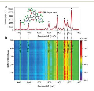
Fig. 4 (a) Average SERS spectra measured from the R6G-treated 3D Ag hybrid nanostructure under the excitation laser wavelength of 473 nm. The concentration of R6G used in the measurement is  $10^{-7}$  M. (b) SERS contour plot of R6G (10<sup>-7</sup> M) on the R6G-treated 3D-Ag-HNA substrate at 50 different locations.
