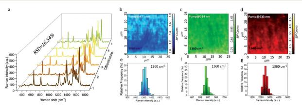
Fig. 7 (a) SERS spectra of 10<sup>-7</sup> M R6G collected from six 3D-Aq-HNA substrates of different batches. Raman intensity spatial distribution of the R6G 1360 cm<sup>-1</sup> band over the mapping area obtained at the excitation wavelength of (b) 473 nm, (c) 514 nm and (d) 633 nm. Histograms of Raman intensities at 1360 cm<sup>-1</sup> under different laser excitations: (e) 473 nm, (f) 514 nm and (g) 633 nm.
