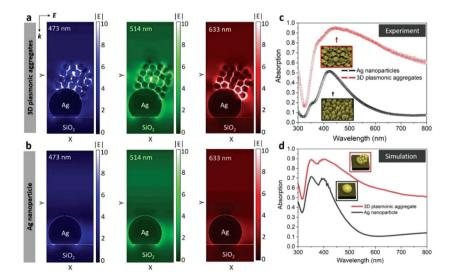
Fig. 3 Simulated electric field distribution of 3D Ag HNA (a) and conventional Ag NPs (b) under different excitation wavelengths (473 nm, 514 nm and 633 nm). Experimental (c) and simulated (d) optical absorption of the large size Ag NPs and the 3D-HNAs.
