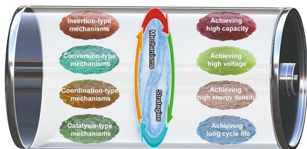
Fig. 2 Overview of energy storage mechanisms and design strategies employed in Zn-based battery systems.
