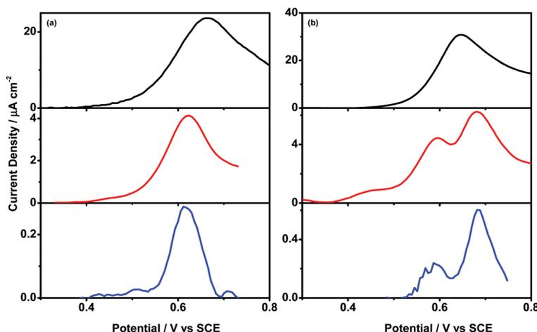
**Fig. 3** Differential pulse voltammetry of: (a) ITC  $10^{-4}$  M (black line),  $10^{-5}$  M (red line) and  $10^{-6}$  M (blue line) in pH 9 buffer + 0.1 NaCl; and (b) SUN  $10^{-4}$  M (black line),  $10^{-5}$  M (red line) and  $10^{-6}$  M (blue line) in pH 7 buffer + 0.1 NaCl on the GC electrode.
