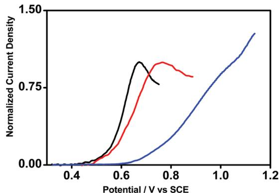
Fig. 1 Normalized single sweep cyclic voltammograms of ITC  $10^{-4}$  M in pH 9 buffer + NaCl 0.1 M at: ITO (blue line), ITO/NT (black line) and GC (red line) electrodes.  $v = 0.02$  V s<sup>-1</sup>.
