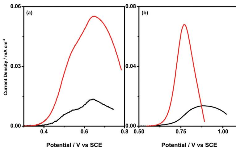
**Fig. 2** Single sweep cyclic voltammograms of: (a) SUN  $4 \times 10^{-5} \text{ M}$  in 1:3 v DMSO/water pH 9 buffer + 0.1 NaCl at GC (black line) and GC/NafionNT (red line) electrodes, and (b) ITC  $10^{-4} \text{ M}$  in pH 9 buffer + NaCl 0.1 M at GC (black line) and GC/PEDOT (red line) electrodes.  $v = 0.02 \text{ V s}^{-1}$ .
