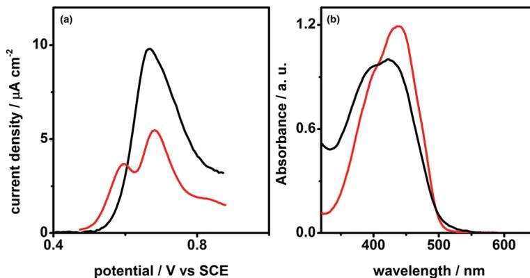
Fig. 4 (a) Differential pulse voltammetry of SUN  $10^{-5}$  M in pH 7 buffer + 0.1 NaCl with 25% DMSO (black line) and 2.5% DMSO (red line) at the CG electrode. (b) UV-vis spectra of SUN  $10^{-5}$  M in water (black line) and in 1:3 v/v DMSO/water mixture (red line).
