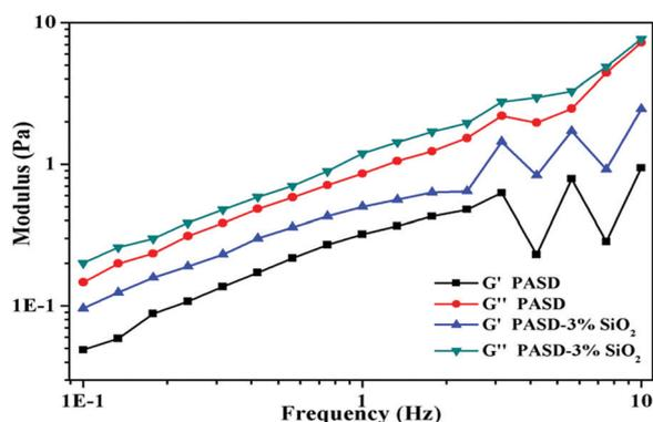
Fig. 13 Storage moduli and loss moduli as a function of frequency for PASD and PASD-3%SiO<sub>2</sub>.
