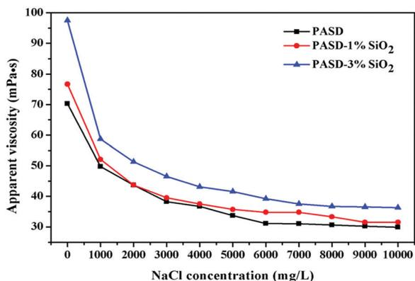
Fig. 10 Effect of the NaCl concentration on apparent viscosity of PASD and PASD-SiO<sub>2</sub>.
