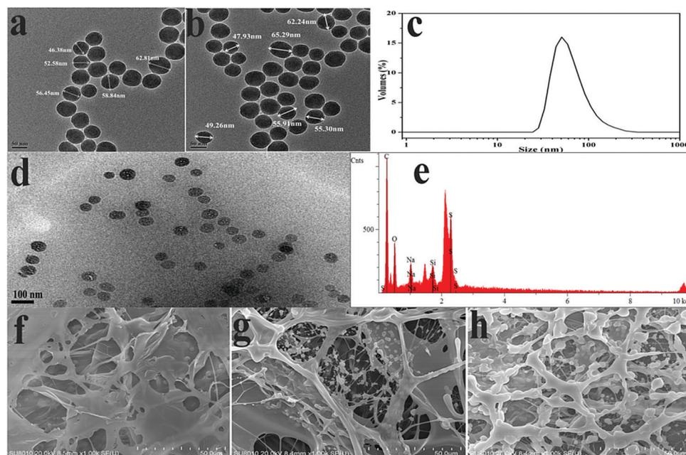
Fig. 6 TEM micrographs of (a) pure  $\text{SiO}_2$  and (b) modified  $\text{SiO}_2$ , (c) particle size distribution of modified  $\text{SiO}_2$ , (d) TEM image of PASD-2% $\text{SiO}_2$ , (e) elemental analysis of PASD-3% $\text{SiO}_2$ , SEM images of (f) 0.5 wt% PASD, (g) 0.5 wt% PASD-2% $\text{SiO}_2$  and (h) 0.5 wt% PASD-3% $\text{SiO}_2$ .
