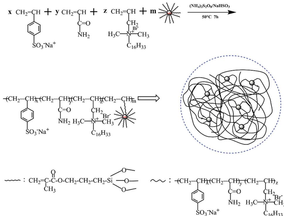
Fig. 3 Chemical route to the synthesis of PASD-SiO<sub>2</sub>.
