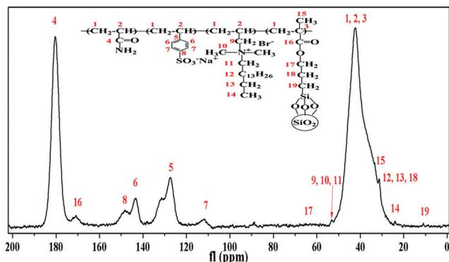
Fig. 5  $^{13}\text{C}$ -NMR spectra of PASD-3% $\text{SiO}_2$ .
