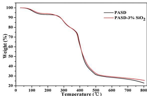
Fig. 8 Thermal gravimetric curves of PASD and PASD-3%SiO<sub>2</sub>.
