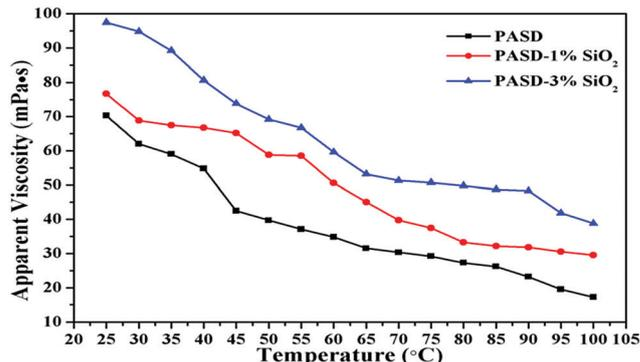
Fig. 11 Apparent viscosity of PASD, PASD-1%SiO<sub>2</sub> and PASD-3%SiO<sub>2</sub> as a function of temperature.
