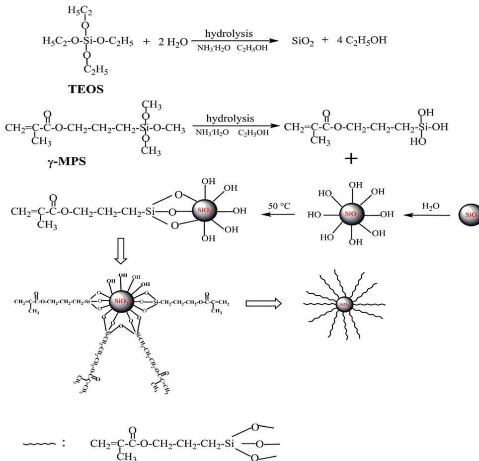
Fig. 1 Chemical route to the modified nanosilica.
