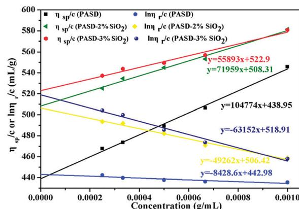
Fig. 9 Intrinsic viscosity of PASD and PASD-SiO<sub>2</sub> vs. concentration.
