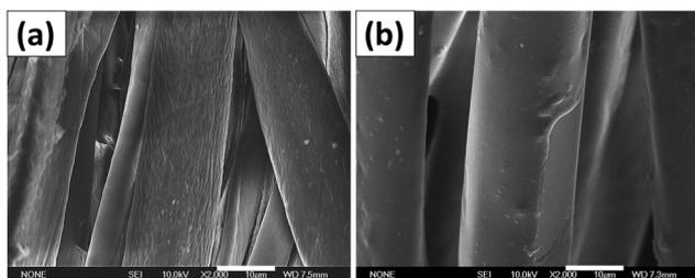
**Fig. 10** SEM micrographs of polyester fabrics (a) and fabrics coated with D<sub>2</sub>WPU (b). The scale bars are 10 µm.
