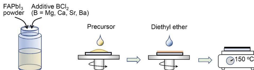
**Fig. 1** A schematic illustration of the perovskite deposition procedure. The precursor solution was prepared by mixing the pre-synthesized FAPbI<sub>3</sub> powder with BCl<sub>2</sub> additive (B = Mg, Ca, Sr and Ba), which was spin-coated. Diethyl ether was dripped for 20 s after rotating the substrate. The film was annealed at 150 °C in an air atmosphere.
