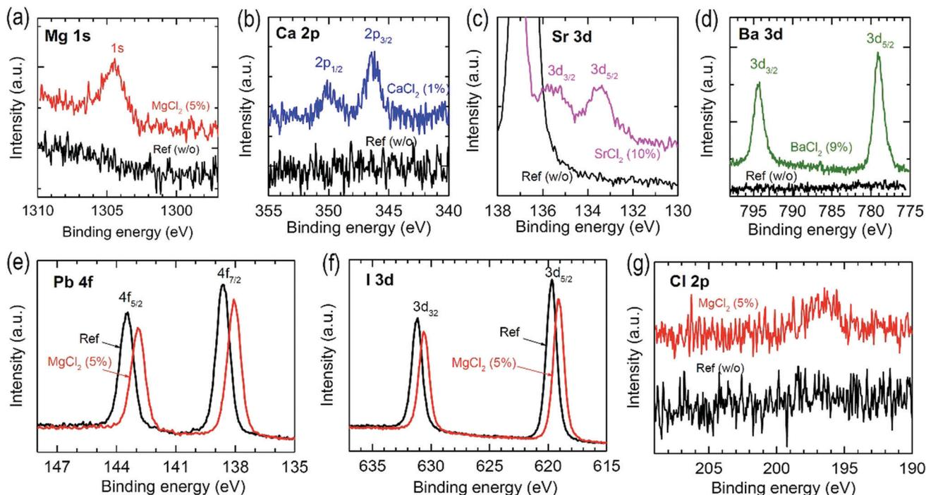
Fig. 5 Mg 1s, Ca 2p, Sr 3d and Ba 3d X-ray photoelectron spectroscopy (XPS) spectra of the annealed FAPbI<sub>3</sub> films with and without additives of (a) MgCl<sub>2</sub>, (b) CaCl<sub>2</sub>, (c) SrCl<sub>2</sub> and (d) BaCl<sub>2</sub>. (e) Pb 4f, (f) I 3d and (g) Cl 2p XPS spectra of the FAPbI<sub>3</sub> films before and after adding the MgCl<sub>2</sub> additive.
