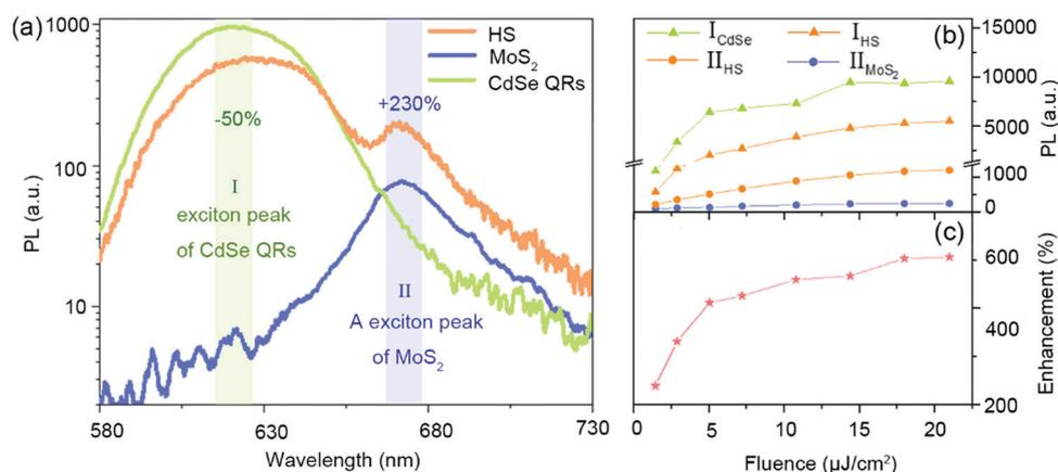
Fig. 2 (a) PL spectra of heterostructure (orange), pristine MoS<sub>2</sub> monolayer (blue), and CdSe QRs (green). (b) PL intensity of all of the heterostructure, MoS<sub>2</sub>, and CdSe QRs. (c) PL enhancement of MoS<sub>2</sub> as a function of incident fluence. Defining  $I_{HS}/I_{MoS_2}$  as PL enhancement.
