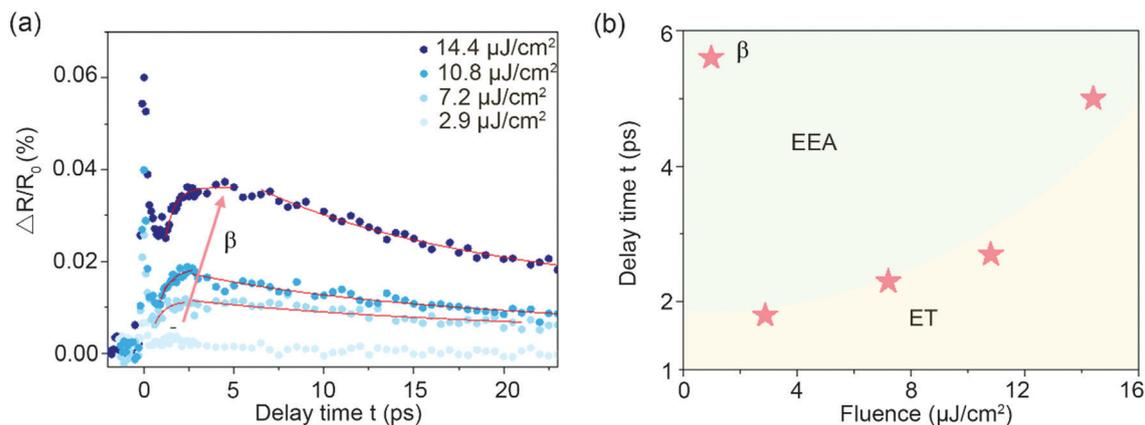
Fig. 4 (a) Time-resolved transient differential reflection spectra of the heterostructure as a function of pump fluence. (b) The appearance time of point  $\beta$  as a function of pump fluence. The area with a yellow background indicates that energy transfer dominates exciton relaxation, while the area with a green background implies that exciton relaxation is dominated by EEA.
