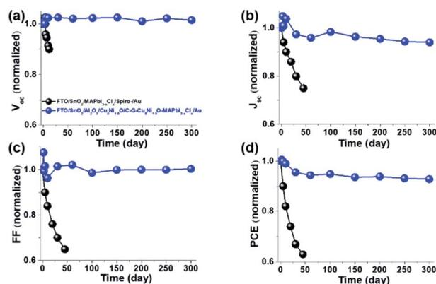
Fig. 4 Long-term stability of FTO/SnO<sub>2</sub>/MAPbI<sub>3-x</sub>Cl<sub>x</sub>/spiro-OMeTAD/Au (black) and FTO/SnO<sub>2</sub>/Al<sub>2</sub>O<sub>3</sub>/Cu<sub>δ</sub>Ni<sub>1-δ</sub>O/C-G-Cu<sub>δ</sub>Ni<sub>1-δ</sub>O-MAPbI<sub>3-x</sub>Cl<sub>x</sub>/Au under ambient conditions (45–50% humidity and 25–30 °C).
