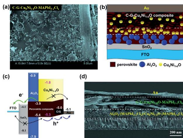
Fig. 1 (a) The surface morphology of the C-G-Cu<sub>δ</sub>Ni<sub>1-δ</sub>O-MAPbI<sub>3-x</sub>Cl<sub>x</sub> composite film, (b) device configuration, (c) schematic of the energy band diagram and blocking properties and (d) a cross-sectional SEM image for HCF-PSCs of FTO/SnO<sub>2</sub>/Al<sub>2</sub>O<sub>3</sub>/Cu<sub>δ</sub>Ni<sub>1-δ</sub>O/C-G-Cu<sub>δ</sub>Ni<sub>1-δ</sub>O-MAPbI<sub>3-x</sub>Cl<sub>x</sub>/Au.
