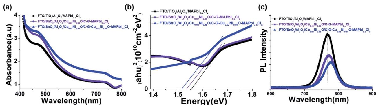
**Fig. 2** (a) UV-vis spectra, (b) corresponding Tauc plots and (c) PL spectra for three films: FTO/TiO<sub>2</sub>/Al<sub>2</sub>O<sub>3</sub>/MAPbI<sub>3-x</sub>Cl<sub>x</sub> (dark), FTO/SnO<sub>2</sub>/Al<sub>2</sub>O<sub>3</sub>/Cu<sub>δ</sub>Ni<sub>1-δ</sub>O/C-G-MAPbI<sub>3-x</sub>Cl<sub>x</sub> (purple) and FTO/SnO<sub>2</sub>/Al<sub>2</sub>O<sub>3</sub>/Cu<sub>δ</sub>Ni<sub>1-δ</sub>O/C-G-Cu<sub>δ</sub>Ni<sub>1-δ</sub>O-MAPbI<sub>3-x</sub>Cl<sub>x</sub> (blue).
