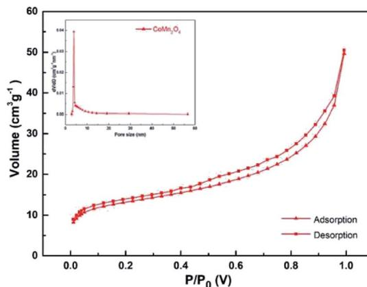
Fig. 6  $\text{N}_2$  adsorption/desorption isotherms of  $\text{CoMn}_2\text{O}_4$ .
