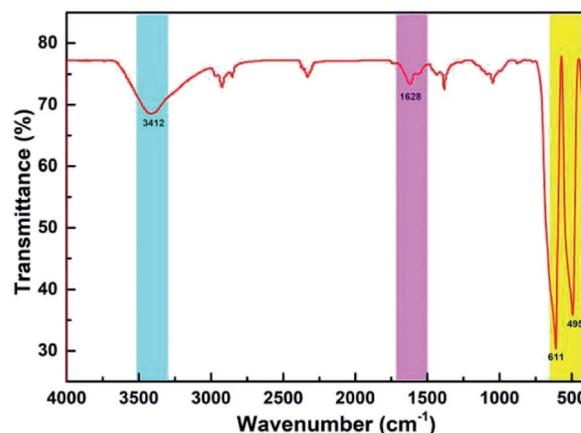
Fig. 2 Fourier transform infrared (FT-IR) spectra of  $\text{CoMn}_2\text{O}_4$ .
