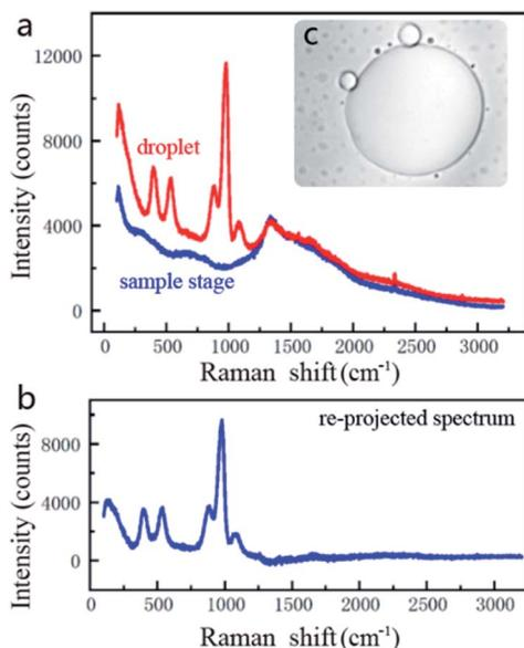
**Fig. 2** Raw spectra measured by using a Raman spectrometer and the processed spectrum of droplets. (a) The red line is a typical raw spectrum of droplets and the blue line is the signal of the sample chamber. (b) is the re-projected spectrum obtained by subtracting the spectrum of the sample chamber from the droplets' waveform. (c) Shows the large droplet attached on the coverslip.
