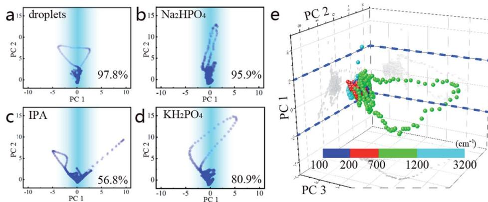
Fig. 4 The analysis results of PCA in different dimensions. PC  $n$  represents the distribution of all data relative to the principal component  $x$ . (a–d) are the PCA between the spectra of dried droplets and normal droplets,  $\text{Na}_2\text{HPO}_4$ , IPA, and  $\text{KH}_2\text{PO}_4$ , separately. (e) is a routine PCA of droplets and all components of PBS.
