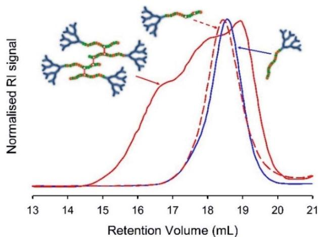
**Fig. 4** Illustrative example of TD-SEC analysis (refractive index) of pH-triggered degradation of BDME containing hyperbranched-polydendrons. Example shows statistical *hyp*-PD  $G_2-p(\text{DEAEMA}_{33}\text{-co-HPMA}_{17}\text{-co-BDME}_{2,0})$  before addition of HCl (red solid line), the sample after acid addition and purification (red dotted line) and the corresponding  $G_2-p(\text{DEAEMA}_{33}\text{-co-HPMA}_{17})$  statistical linear-dendritic hybrid (blue solid line) for comparison.
