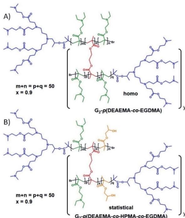
Fig. 2 Homo and statistical hyperbranched-polydendron chemical structure examples using the  $G_2$  amine functional dendron initiator, **1**. (A) Homo *hyp*-PD comprising poly(2-(diethyl amino)ethyl methacrylate), DEAEMA, within the primary chains using ethylene glycol dimethacrylate, EGDMA, as the branching agent; (B) statistical *hyp*-PD comprising DEAEMA, EGDMA and 2-hydroxy propyl methacrylate within the primary chains.
