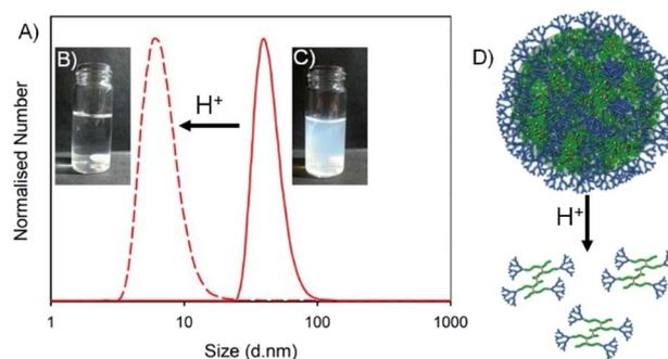
Fig. 6 Example of pH-response for nanoprecipitates formed from  $G_2$ -*p*(DEAEMA<sub>50</sub>-*co*-EGDMA<sub>0,9</sub>). (A) Impact of added HCl to aqueous dispersion of nanoparticles ( $D_n$  distribution shown); (B and C) visual impact of addition of HCl to the nanoprecipitate dispersion; (D) schematic representation of the disassembly of nanoprecipitates to component solvated hyperbranched-polydendrons.
