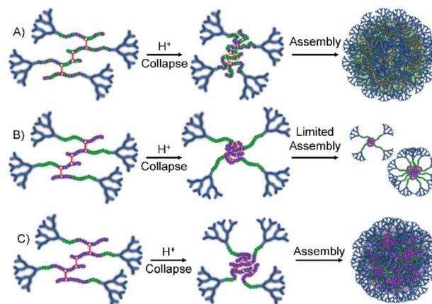
**Fig. 5** Schematic representation of the behaviour of statistical and block hyperbranched-polydendrons containing varying  $t$ -butyl methacrylate ( $t$ BuMA) monomer residue content during nanoprecipitation into acidic water. (A) Statistical  $hyp$ -PD with high  $t$ BuMA content; (B) block  $hyp$ -PD with short  $t$ BuMA block length; (C) block  $hyp$ -PD with long  $t$ BuMA block length.
