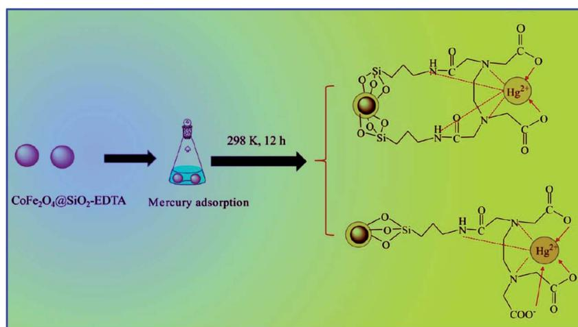
Fig. 16 Schematic of the mechanism of the adsorption of Hg<sup>2+</sup> by magnetic CoFe<sub>2</sub>O<sub>4</sub>@SiO<sub>2</sub>-EDTA adsorbent (ref. 183).
