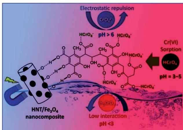
Fig. 12 Schematic representation of the adsorption of chromium ions by the HNT/ $\text{Fe}_3\text{O}_4$ -HA nanoadsorbent at different pH. (Reprinted with permission from ref. 140, Copyright © (2020) John Wiley and Sons.)
