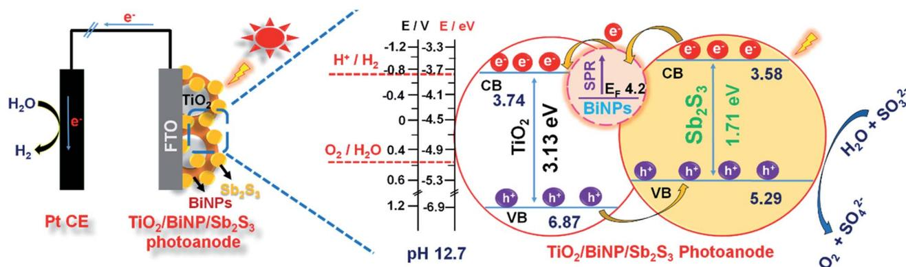
Fig. 5 A scheme of a PEC cell constructed using the ternary photoanode  $\text{TiO}_2/\text{BiNP}/\text{Sb}_2\text{S}_3$ , showing the band alignment, charge transport and redox reactions under the simulated solar irradiation.
