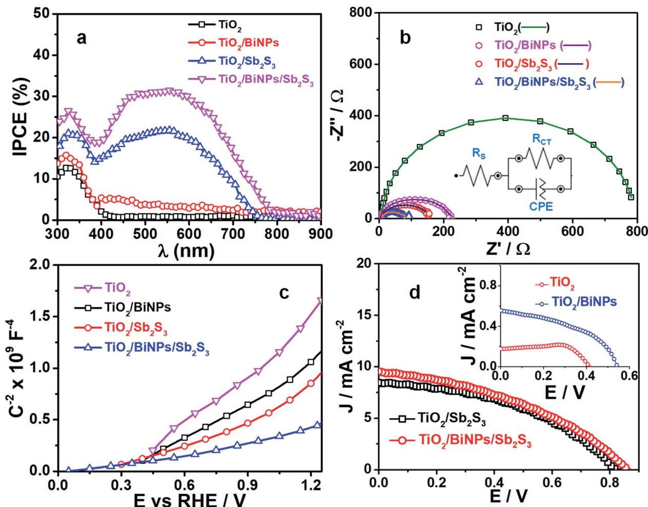
Fig. 4 IPCE and  $I/V/R$  characteristics of photoanodes. (a) Wavelength-dependent IPCE plots (b) Nyquist plots (symbol) with an equivalent circuit (dot lines) and (c) Mott–Schottky plots of pristine  $\text{TiO}_2$ ,  $\text{TiO}_2/\text{BiNP}$ ,  $\text{TiO}_2/\text{Sb}_2\text{S}_3$  and  $\text{TiO}_2/\text{BiNP}/\text{Sb}_2\text{S}_3$  photoanodes. (d)  $J-V$  data of  $\text{TiO}_2/\text{Sb}_2\text{S}_3$  and  $\text{TiO}_2/\text{BiNP}/\text{Sb}_2\text{S}_3$  photoanodes.
