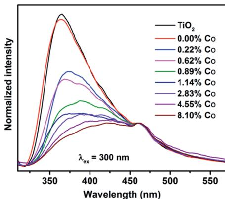
Fig. 5 Emission spectra of undoped and  $\text{Co}_{(\text{doped})}\text{-TiO}_2$  nanocrystals ( $\lambda_{\text{ex}} = 300$  nm). The weak feature at 460 nm is an artifact due to scattering of light from the Xe lamp; all spectra were normalized to the intensity of the artifact.
