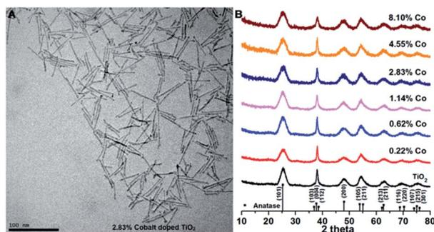
Fig. 3 (A) TEM image of  $\text{Co}_{(\text{doped})}\text{-TiO}_2$  nanocrystals (cobalt analysis = 2.83%; others are shown in Fig. S2†); (B) powder X-ray diffraction pattern of  $\text{Co}^{2+}_{(\text{doped})}\text{-TiO}_2$  nanocrystals at different cobalt concentration.
