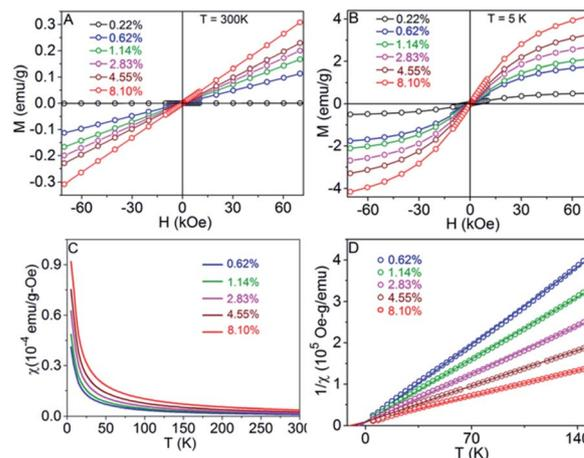
Fig. 9 Magnetic properties of Co-doped  $\text{TiO}_2$  nanocrystals for different wt% of Co: field-dependent magnetization curves measured at 300 K (A) and 5 K (B). (C) Temperature-dependent susceptibility. (D) The inverse susceptibility is fitted using Curie–Weiss expression, where the open circles correspond to the experimental data and solid lines represent fitting results.
