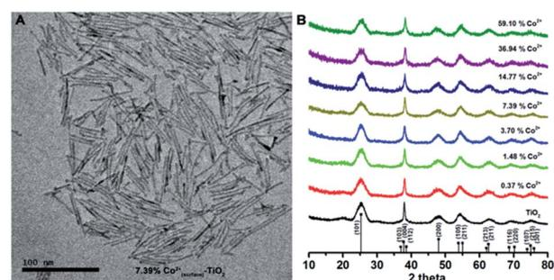
Fig. 2 (A) TEM image of Co<sup>2+</sup><sub>(surface)</sub>-TiO<sub>2</sub> nanorods (Co analysis = 7.4%; others are shown in Fig. S1†); (B) powder X-ray diffraction pattern of Co<sup>2+</sup><sub>(surface)</sub>-TiO<sub>2</sub> nanorods.
