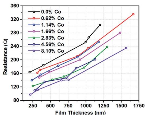
Fig. 8 Resistance versus film thickness for thin-film samples of  $\text{Co}_{(\text{doped})}\text{-TiO}_2$  on ITO-coated glass substrate.
