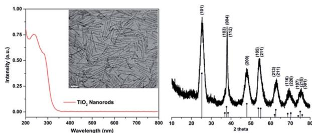
Fig. 1 Left: UV-visible absorption spectrum of TiO<sub>2</sub> nanorods; left (inset): transmission electron micrograph of TiO<sub>2</sub> nanorods (scale bar = 20 nm); right: powder X-ray diffraction pattern of TiO<sub>2</sub> nanorods.
