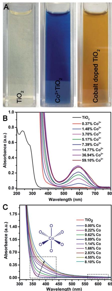
Fig. 4 (A) Photograph of (left)  $\text{TiO}_2$  nanorods dispersed in hexanes, (middle)  $\text{Co}^{2+}_{(\text{surface})}\text{-TiO}_2$  nanorods dispersed in hexanes, and (right)  $\text{Co}_{(\text{doped})}\text{-TiO}_2$  nanorods dispersed in hexanes; (B) UV-visible absorption spectra of  $\text{Co}^{2+}_{(\text{surface})}\text{-TiO}_2$  nanocrystals; (C) UV-visible absorption spectra of  $\text{Co}_{(\text{doped})}\text{-TiO}_2$  nanocrystals.
