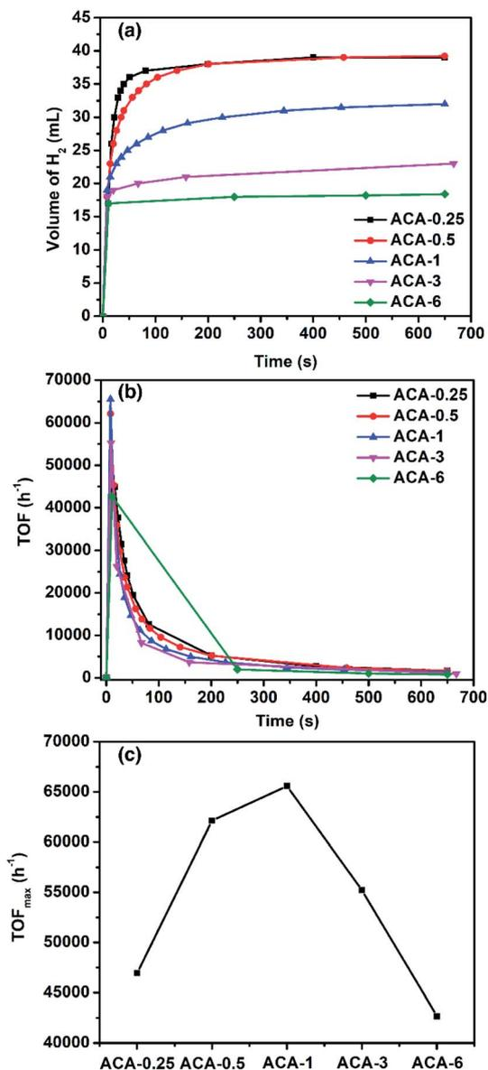
Fig. 4 (a) Volume of H<sub>2</sub> produced as a function of time for various ACA catalysts. Here 2 : 1 molar ratio of ammonia borane to sodium borohydride (10 mg ammonia borane and 6.2 mg sodium borohydride) was dissolved in 2 mL water and added to 50 mg of ACA-1, which was stirred at 735 rpm. (b) TOF as a function of time for various ACA catalysts. (c) The TOF<sub>max</sub> obtained for various ACA catalysts.
