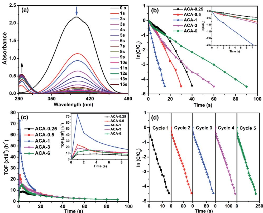
Fig. 3 (a) Time-resolved UV-visible spectral profiles of 4-nitrophenol reduction with sodium borohydride in the presence of the ACA-1 catalyst. (b) Plot of  $\ln(C/C_0)$  versus time for all ACA samples for the benchmark 4-nitrophenol reduction reaction (the amount of gold was maintained the same in all reactions). (c) Plot of TOF as a function of reaction time for the corresponding data in (b). (d) Cyclability studies up to 5 cycles of 4-nitrophenol reduction using the ACA-1 catalyst.
