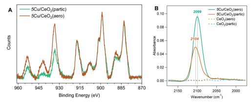
Fig. 5 (A) Background-subtracted X-ray photoelectron spectra of 5Cu/CeO<sub>2</sub>(partic) (amber) and 5Cu/CeO<sub>2</sub>(aero) (green) in the Ce 3d (875 to 925 eV) and Cu 2p (925 to 965 eV) regions. (B) ATR-FTIR spectra for 5Cu/CeO2(aero) (green), 5Cu/CeO2(partic) (amber), CeO2(aero) (dashed yellow), and CeO<sub>2</sub>(partic) (dashed blue), showing CO binding at 2099 cm<sup>-1</sup> and 2104 cm<sup>-1</sup> for 5Cu/CeO<sub>2</sub>(aero) and 5Cu/CeO<sub>2</sub>(partic), respectively.
