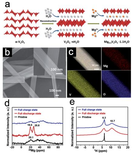
Fig. 3 (a) Schematic of the formation of the  $Mg_{0.3}V_2O_5\cdot 1.1H_2O$  nanowires. (b) SEM images and (c) TEM-EDX element mapping images of  $Mg_{0.3}V_2O_5\cdot 1.1H_2O$  nanowires. (d)  $^{25}Mg$  (D) and (e)  $^{1}H$  (E) MAS NMR spectra collected for  $Mg_{0.3}V_2O_5\cdot 1.1H_2O$  in different states. Panels reproduced with permission. Copyright 2019, Elsevier.
