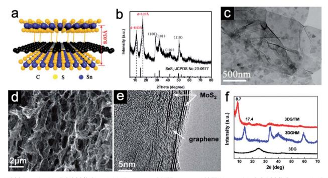
Fig. 2 (a) Schematic of the  $SnS_2/rGO/SnS_2$  sandwich-like structure. (b) XRD pattern and (c) TEM image of the  $SnS_2/rGO/SnS_2$  composite. Panels (a-c) reproduced with permission.<sup>40</sup> Copyright 2019, American Chemical Society. (d) SEM image of the porous 3DG/TM. (e) HRTEM image of 3DG/TM. (f) XRD patterns of 3DG/TM and control samples. Panels (d-f) reproduced with perpission. 41 Copyright 2019, The Royal Society of Chemistry.
