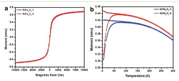
Fig. 4 (a) Magnetic hysteresis curves (Mvs. H) of samples NiFe<sub>2</sub>O<sub>4</sub>-3 and NiFe<sub>2</sub>O<sub>4</sub>-4 at 300 K and (b) temperature dependence of magnetization of samples NiFe<sub>2</sub>O<sub>4</sub>-3 and NiFe<sub>2</sub>O<sub>4</sub>-4 measured under field-cooled (FC) and zero-field-cooled (ZFC) conditions at an applied field of 500 Oe.
