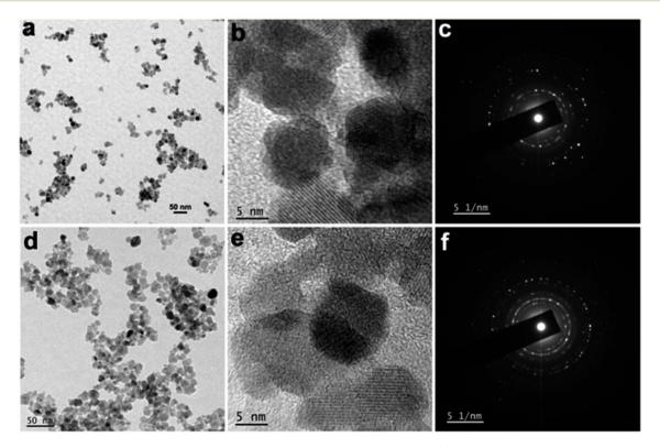
Fig. 3 TEM images of the as-prepared NiFe<sub>2</sub>O<sub>4</sub> NPs: (a) TEM image, (b) HRTEM image, and (c) SAED pattern recorded from sample NiFe<sub>2</sub>O<sub>4</sub>-3 and (d) TEM image, (e) HRTEM image, and (f) SAED pattern recorded from sample NiFe<sub>2</sub>O<sub>4</sub>-4.
