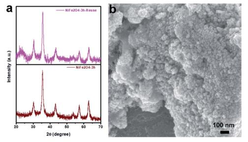
Fig. 7 (a) XRD pattern and (b) SEM image of the recovered NiFe<sub>2</sub>O<sub>4</sub> NPs after catalysis.
