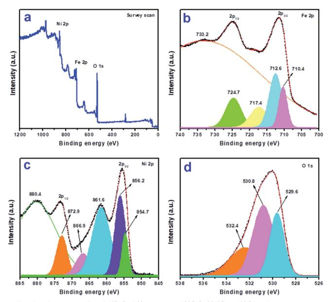
X-ray photoelectron spectra of sample NiFe<sub>2</sub>O<sub>4</sub>-4: (a) survey scan, and (b) Fe 2p, (c) Ni 2p, and (d) O 1s regions.
