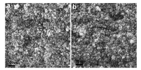
Fig. 2 FESEM images of the as-prepared NiFe<sub>2</sub>O<sub>4</sub> NPs: (a) sample NiFe<sub>2</sub>O<sub>4</sub>-3 and (b) sample NiFe<sub>2</sub>O<sub>4</sub>-4
