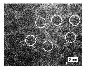
Fig. 1  $\,$  TEM image of colloidal CdSe NCs. The white circles indicate single CdSe NCs for clarity.
