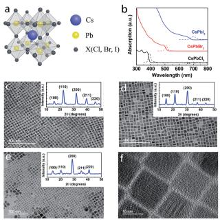
Fig. 1 Structural characterization of CsPbX<sub>3</sub> nanocrystals (NCs). (a) A schematic crystal structure of a cubic CsPbX<sub>3</sub> perovskite. (b) Room temperature absorption (solid) and PL spectra (dashed) of CsPbX<sub>3</sub> NCs in a hexane solution. TEM images of (c) CsPbCl<sub>3</sub>, (d) CsPbBr<sub>3</sub>, and (e) CsPbI<sub>3</sub> NCs. (f) High-resolution TEM image of CsPbI<sub>3</sub> NCs. The insets in panels (c-e) are the corresponding room temperature XRD patterns.
