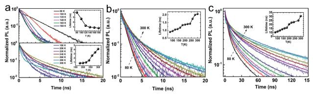
Fig. 3 TRPL characteristics of CsPbX<sub>3</sub> NCs. Normalized TRPL data of (a) CsPbCl<sub>3</sub>, (b) CsPbBr<sub>3</sub>, and (c) CsPbI<sub>3</sub> NCs in the temperature range from 80-300 K. Each colored trace in the figure represents TRPL data that were collected at a specific temperature (legends shown in panel (a)). The solid traces are fits to the data, and the insets show the corresponding lifetimes. For clarity, two sub-panels are shown in panel (a).
