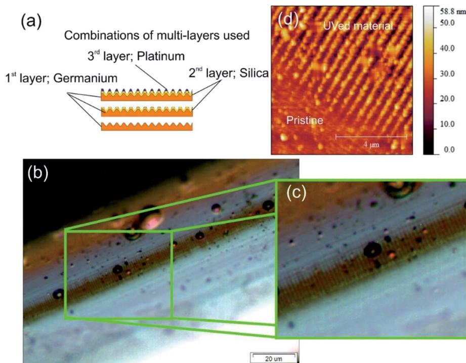
Fig. 2 (a) The fabrication procedure and materials used ( $\text{Ge}-\text{SiO}_2-\text{Pt}$ ) and appearance of the plasmonic devices. (b and c) A microscope image of a section of coated (coating  $\text{Ge}-\text{SiO}_2-\text{Pt}$ ) D-shaped fibre that has been UV processed, with a magnified inset to show the surface corrugation. (d) An AFM topographical map showing a typical surface of the material before and after UV exposure (germanium, silicon dioxide, platinum).
