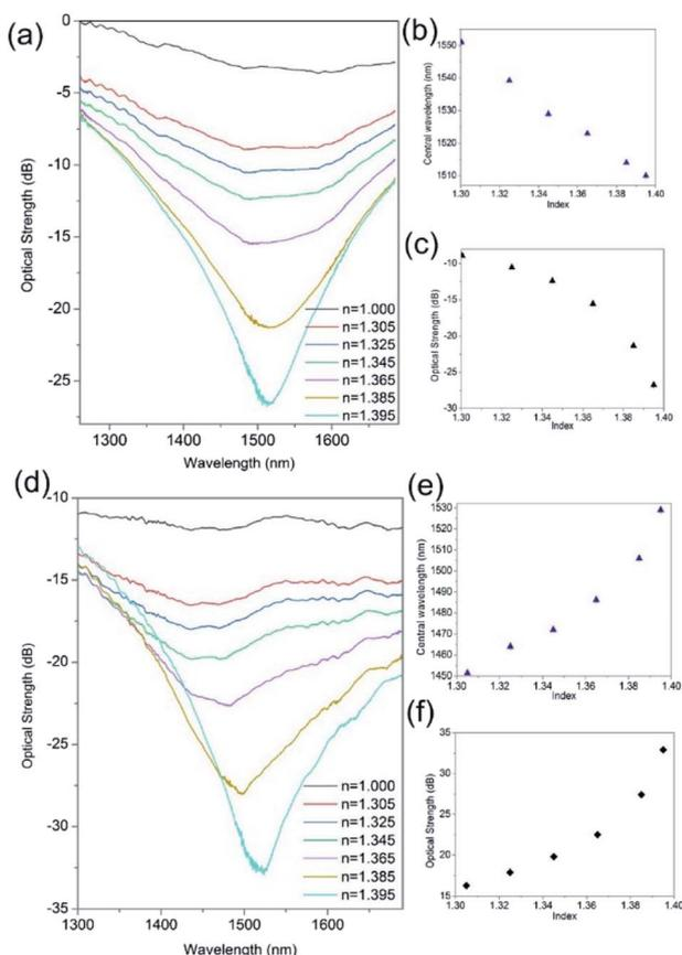
Fig. 4 An example of the variation in refractive index sensitivity of a Ge/SiO<sub>2</sub>/Pt fibre plasmonic device. Before UV processing (a) the transmission spectra as a function of index, (b) central wavelength (c) optical coupling strength. After UV processing (d) the transmission spectra as a function of index, (e) central wavelength (f) optical coupling strength.
