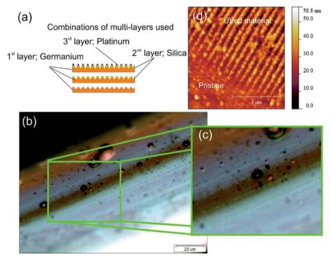
Fig. 2 (a) The fabrication procedure and materials used ( $Ge-SiO_2-Pt$ ) and appearance of the plasmonic devices. (b and c) A microscope image of a section of coated (coating  $Ge-SiO_2-Pt$ ) D-shaped fibre that has been UV processed, with a magnified inset to show the surface corrugation. (d) An AFM topological map showing a typical surface of the material before and after UV exposure (germanium, silicon dioxide, platinum).
