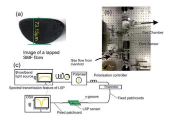
Fig. 1 (a) Microscope image of the cross-section of the D-shaped fibre used in the fabrication process. (b) The gas chamber used to replace the V-groove for refractive index sensitivity in the gaseous regime. (c) A general schematic of the characterisation apparatus used.
