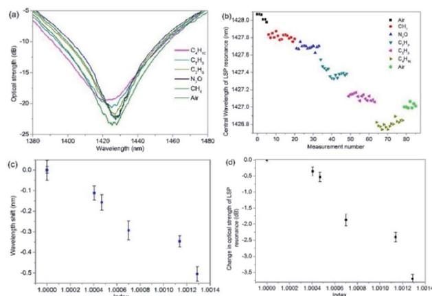
Fig. 5 Typical experimental gas index regime results with UV processed Ge/SiO<sub>2</sub>/Pt device (a) the transmission spectra as a function of different gases (b) the individual measurements of the central wavelength of the LSP resonance for each gas from the experiments. (c and d) The wavelength and optical strength sensitivity as a function of the different refractive indices of the alkane gases and nitrous oxide, respectively.
