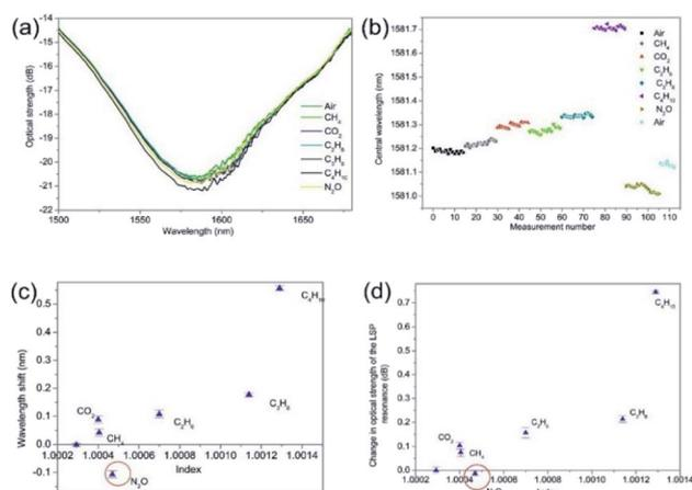
Fig. 6 Typical experimental results of an UVed  $\text{Ge}/\text{SiO}_2/\text{Pt}$  LSP fibre device coated with SWNTs as a function of surrounding refractive index and nitrous oxide (a) the transmission spectra as function of surrounding gas. (b) The individual measurements of the central wavelength of the LSP resonance for each alkane gas and nitrous oxide (c) and (d) the wavelength and optical strength sensitivity as a function of the different gas's refractive index respectively.
