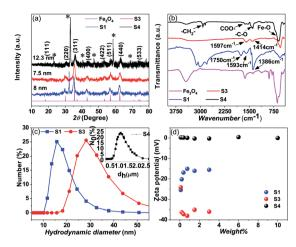
Fig. 2 (a) XRD pattern of the prepared magnetite samples S1, S3 and S4, (b) FTIR vibration band spectra for samples S1, S3, S4 and  $Fe_3O_4$ , (c) DLS of the synthesized samples S1 and S3, and (d) zeta potential measurement for different weight percentages of magnetite nanoparticles of samples S1, S3 and S4.
