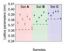
Fig. 8 Lattice parameters measured from electron diffraction patterns on different sets of particles in samples A, B and C compared to reference values in the corresponding bulk materials (dashed straight line).
