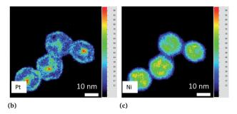
Fig. 1 Ni<sub>3</sub>Pt colloidal synthesis performed at 225 °C. (a) STEM-HAADF image and chemical mappings using EDX mode with the concentration scale demonstrate that (b) Pt ( $L_{\alpha}$  line) is predominantly located in the core and (c) Ni ( $K_{\alpha}$  line) mainly in the shell.
