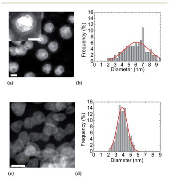
Fig. 4 STEM-HAADF micrographies and size distribution histograms of Ni $_3$ Pt NPs elaborated at (a and b) 200 °C showing a core-shell structure and an observable organic layer surrounding the particle in the magnified image in the inset and at (c and d) 280 °C showing alloyed particles (scale bar = 5 nm).
