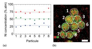
Fig. 6 (a) Chemical composition distribution extracted from EDX chemical mappings recorded on isolated NPs in samples A (in red), B (in green) and C (in blue). (b) Example of a chemical mapping sampling of 8 NPs in sample B with Ni in red and Pt in green (scale bar = 5 nm).
