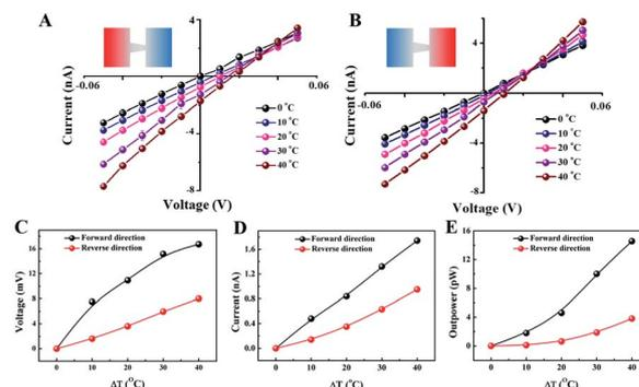
Fig. 3 Theoretical thermometric conversion capability. The base side was repositioned towards the cold side or hot side. (A) The  $I$ - $V$  curves of the forward direction at different temperature differences and (B) those in the reverse direction. (C) Short-circuit current. (D) Open-circuit voltage. Both were obtained by the intercept of the abscissa and ordinate axes. (E) Outpower calculated by geometric area enclosed by the  $I$ - $V$  curves and coordinate axes.
